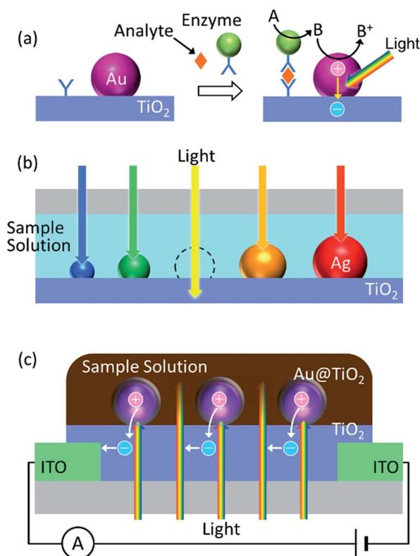
Fig. 10 Chemical sensors and biosensors based on PICS. (a) PICS is used for detection of a marker.<sup>101,102</sup> (b) Dip-based sensor for refractive index sensing.<sup>36</sup> (c) Conductometric sensor for refractive index sensing.<sup>64</sup>
