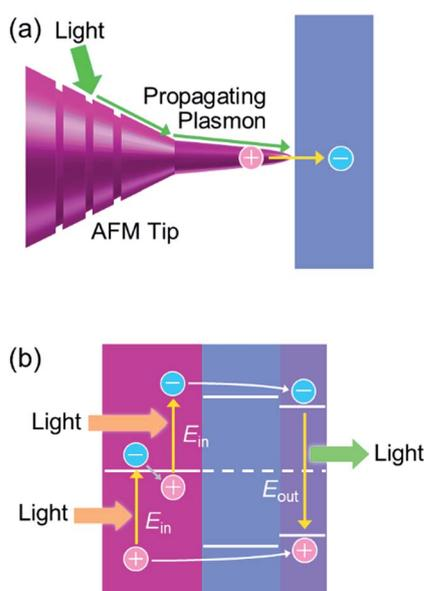
Fig. 12 (a) Scanning-probe nanoscopy<sup>51</sup> and (b) photon upconversion.<sup>119</sup>
