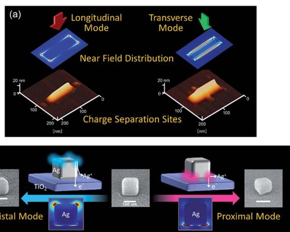
Fig. 7 Results of reaction site analysis for PICS with (a) Ag nanorods on TiO<sub>2</sub> (ref. 58) and (b) Ag nanocubes on TiO<sub>2</sub>.<sup>67</sup> (b) Reproduced with permission from ref. 67 © 2016 American Chemical Society.
