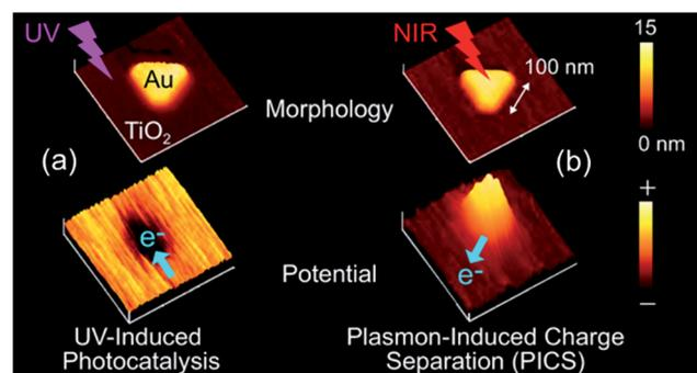
Fig. 6 Results of KFM analysis for the Au nanoplate–TiO<sub>2</sub> system. (Left) The co-catalysis effect and (right) PICS. Reproduced with permission from ref. 60 © John Wiley and Sons.
