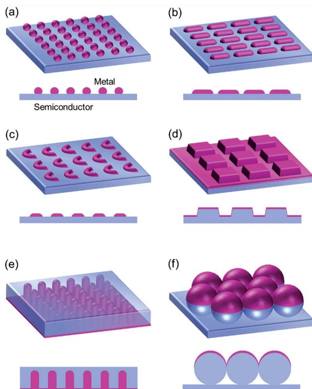
Fig. 9 Metal–semiconductor nanostructure interfaces. (a) Metal nanosphere array, (b) metal nanorod array, (c) chiral metal nanocrescent array, (d) perfect absorber, (e) upright metal nanorod array and (f) metal halfshell array.
