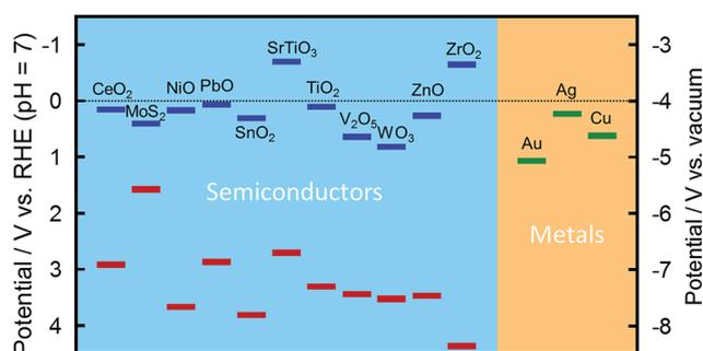
Fig. 4 Positions of the conduction band (blue) and the valence band (red) of selected semiconductors<sup>21–23</sup> and the Fermi level of selected metals.<sup>24</sup>
