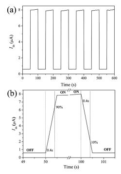
Fig. 7 (a) Time response of the SnS/RGO device illuminated with and without light (100 mW cm $^{-2}$ ). (b) Rise and decay time. All measured at  $V_{\rm ds} = 5.0 \text{ V}, V_{\rm q} = 0 \text{ V}.$
