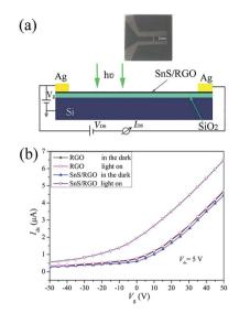
Fig. 4 (a) The optical image and schematic of a representative device. (b) The transfer characteristics  $(l_{\rm ds}-V_{\rm g})$  of the photodetectors based on RGO and SnS/RGO in the dark and under visible-light illumination,  $P=10~{\rm mW~cm^{-2}}$ .
