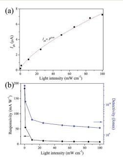
Fig. 6 (a) Plot of photocurrent, (b) corresponding responsivity and detectivity of the device versus light intensities, measured at  $V_{ds}$  = 5.0 V,  $V_{\rm g} = 0$  V.
