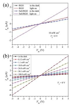
Fig. 5 (a) Output characteristics  $I_{ds}$  –  $V_{ds}$  of the photodetectors based on RGO and SnS/RGO in the dark and under visible-light illumination. (b)  $I_{ds}$ - $V_{ds}$  curves of SnS/RGO with different light intensities.
