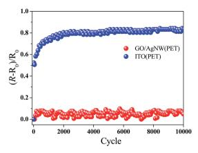
Fig. 6 Variation in the resistance of the GO/AgNW film as a function of the number of bending cycles.
