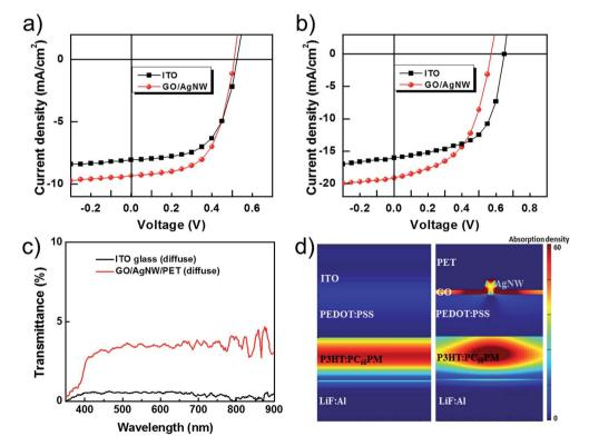
Fig. 7 Representative J-V characteristics of P3HT:PC<sub>60</sub>BM and PTB7:PC<sub>70</sub>BM OSCs with the GO/AgNW mesh electrode and the reference device with the ITO electrode under AM 1.5 G illumination with 100 mW cm<sup>-2</sup> intensity. (a) P3HT:PC<sub>60</sub>BM, (b) PTB7:PC<sub>70</sub>BM. (c) Magnified diffuse transmittance spectra of ITO and GO/AgNW films and (d) simulated light absorption maps in the devices with ITO and GO/AgNW.
