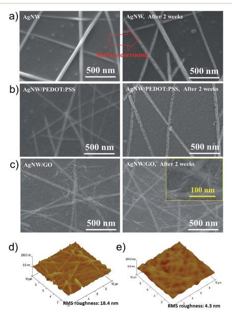
Fig. 4 SEM images of (a) AgNWs and the (b) PEDOT:PSS/AgNW and (c) GO/AgNW hybrid transparent electrodes after a long-term stability test at room temperature for 2 weeks. Atomic force microscopy (AFM) images of AgNWs on PET (d) with and (e) GO/AgNW electrodes.
