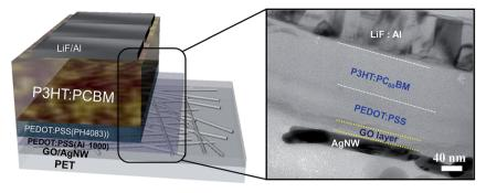
Fig. 2 A schematic cross-sectional view of P3HT:PC<sub>60</sub>BM-based OSCs with GO/AgNW and the corresponding cross-sectional high-resolution transmission electron microscopy (HRTEM) image.
