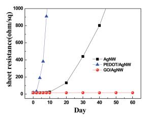
Fig. 5 Plot of the mean  $R_{\rm sh}$  versus time for the AgNW/PET, PEDOT:PSS/ AgNW/PET and GO/AgNW/PET films exposed to air up to 2 months.
