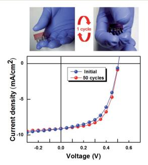
Fig. 8 Photographs of the continuous mechanical bending experiment of a P3HT:PC<sub>60</sub>BM OSC with the GO/AgNW mesh and selected J-V characteristics during bending cycles up to 50.
