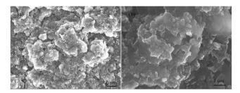
Fig. 4 Ex situ SEM images of the  $CoS_2/G$  electrode after 100 cycles at a current density of 500 mA g<sup>-1</sup>: (a) low magnification, and (b) high magnification.
