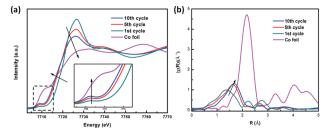
Fig. 7 (a) Ex situ XANES spectra at the Co K-edge of  $CoS_2/G$  at different cycling states. (b) Corresponding ex situ EXAFS spectra.
