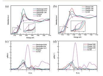
Fig. 6 Ex situ XANES spectra for the Co K-edge of CoS<sub>2</sub>/G at different states: (a) discharge state, and (b) charge state. Corresponding ex situ EXAFS spectra: (c) discharge state, and (d) charge state.
