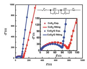
Fig. 5 EIS data of bulk CoS<sub>2</sub> and the CoS<sub>2</sub>/G hybrid composite.
