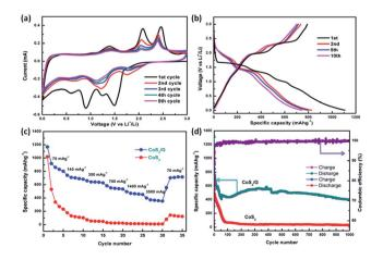
Fig. 3 (a) CV curves of  $CoS_2/G$ , (b) charge–discharge curves of  $CoS_2/G$  at a current density of 70 mA  $g^{-1}$ , (c) rate performance of  $CoS_2/G$  and  $CoS_2$ , and (d) cycle performance with the corresponding coulombic efficiency.
