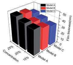
Fig. 6 The film thickness for different asphaltene models at different concentrations
