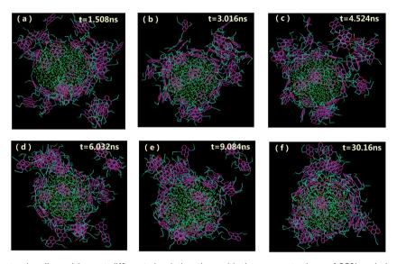
Fig. 3 Morphologies of water-in-oil emulsions at different simulation time with the concentrations of 20% asphaltenes of *Model B*. Different beads in simulations are represented by different colors as can be illustrated from Fig. 1f (the same as below). The toluene molecules are suppressed for clarity.
