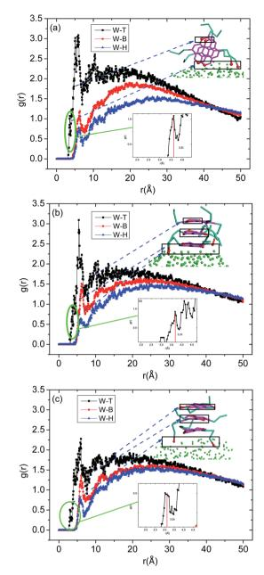
Fig. 8 The radial distribution function *g*(*r*) for different beads in asphaltenes structure including (a) asphaltene molecules of *Model A*, (b) asphaltene molecules of *Model B* and (c) asphaltene molecules of *Model C*. The concentrations of asphaltenes are 20%. The definition of beads can be found in Fig. 1.
