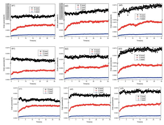
Fig. 9 Order parameter versus simulation the time for different asphaltene models at different concentrations. The asphaltenes of Model A were used: (a1) 15%, (a2) 20%, (a3) 25%; the asphaltenes of Model B were used: (b1) 15%, (b2) 20%, (b3) 25%; the asphaltenes of Model C were used: (c1) 15%. (c2) 20%. (c3) 25%.
