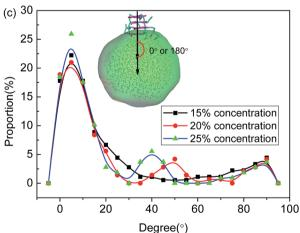
Fig. 5 Temporal evolution of angles between the asphaltene aromatic plane and the O/W interface for the systems including (a) asphaltene molecule of *Model A*, (b) asphaltene molecules of *Model B* and (c) asphaltene molecules of *Model C*. The angle is defined on the basis of the normal of the interface and the normal of the aromatic plane of the island-type asphaltene molecule.
