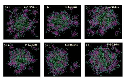
Fig. 2 Morphologies of water-in-oil emulsions at different simulation time with the concentrations of 20% asphaltenes of *Model A*. Different beads in simulations are represented by different colors as can be illustrated from Fig. 1f (the same as below). The toluene molecules are suppressed for clarity.
