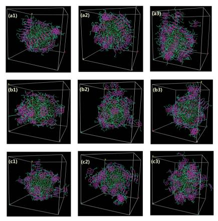
Fig. 4 Morphologies of water-in-oil emulsions at different concentrations with different asphaltene models. Asphaltenes of *Model A* were used: (a1) 15%, (a2) 20%, (a3) 25%; asphaltenes of *Model B* were used: (b1) 15%, (b2) 20%, (b3) 25%; asphaltenes of *Model C* were used: (c1) 15%, (c2) 20%, (c3) 25%. The toluene molecules are suppressed for clarity.
