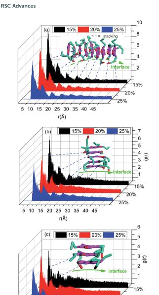
Fig. 7 The radial distribution function g(r) for asphaltenes in different simulation systems including (a) asphaltene molecule of  $Model\ A$ , (b) asphaltene molecules of  $Model\ B$  and (c) asphaltene molecules of  $Model\ C$ .
