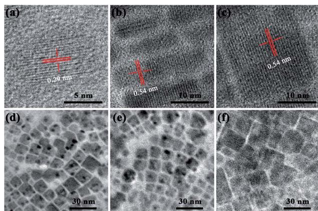
Fig. 1 (a)–(c) Typical HRTEM images of CsPbCl<sub>3</sub> NCs obtained using different reaction conditions. TEM images of cubic CsPbCl<sub>3</sub> NCs after washing (d) two, (e) four, and (f) six times.
