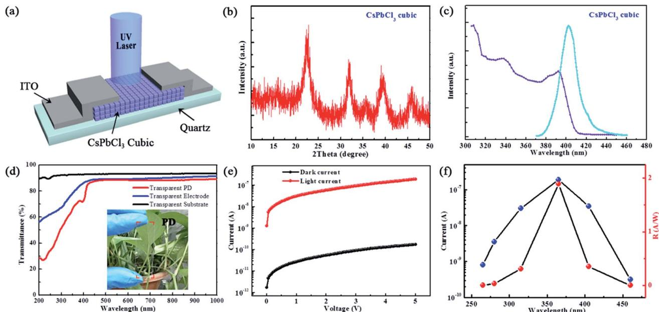
Fig. 3 (a) Schematic of the device. (b) XRD pattern and (c) absorption and emission spectra of cubic CsPbCl<sub>3</sub>. (d) Transmittance spectra of the bare substrate, electrode, and PD device. (e)  $I$ - $V$  logarithm curves of the PD device under 365 nm illumination ( $10 \text{ mW cm}^{-2}$ ) and in darkness. (f) Photocurrent spectrum and  $R$  spectrum of the fabricated PD.
