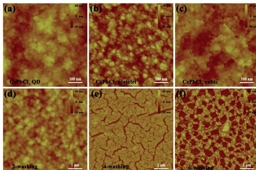
Fig. 2 AFM images of the films fabricated using CsPbCl<sub>3</sub> in (a) QD, (b) platelet, and (c) cubic form. AFM images of the film fabricated using cubic CsPbCl<sub>3</sub> after washing (d) two, (e) four, and (f) six times.
