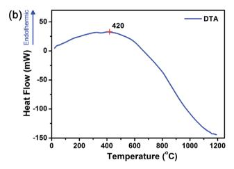
Fig. 2 Simultaneous thermal analysis of the precursor decomposition in inert nitrogen environment shows that there were five transition weight loss transition regions from (a) weight loss profile of the TGA measurements in nitrogen. In addition, precursor decomposition (*i.e.* bond breaking, endothermic) processes dominated at <420 °C and crystallization (*i.e.* bond formation, exothermic) starts from >420 °C from the (b) changes in heat flow based on DTA measurements.
