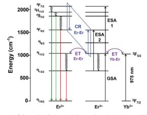
Scheme 3 Schematic of proposed electronic and optical transitions of Gd<sub>2</sub>O<sub>2</sub>S:Yb-Er sub-micron sized particles. ET: energy transfer, CR: cross-relaxation represented by the dashed lines, ESA: excited state absorption, GSA, ground state absorption. Solid arrows represent radiative transitions, whiles the curly arrows represent non-radiative transitions.
