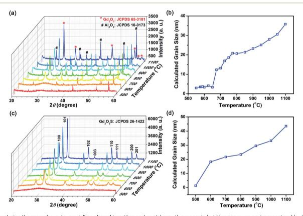
Fig. 3 Analyzing the amorphous-to-crystalline phased transition and crystal growth process in (a, b) inert vacuum environment and (c, d) sulfurrich environment using the XRD. References to JCPDS 65-3181 for  $Gd_2O_3$ , JCPDS 10-0173 for  $Al_2O_3$  and JCPDS 26-1422 for  $Gd_2O_3$ S were used for the phase identification of our samples.  $Al_2O_3$  were identified as present for all samples as the sample holder was made of  $Al_2O_3$  for our quasi in situ XRD measurements.
