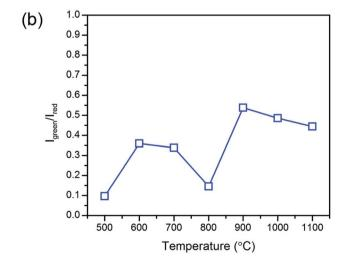
Fig. 5 Heat treatment temperature effects on the upconverted visible and downshifted infrared emissions. The (a) characteristic steady state emission profiles and (b) green-to-red emission intensity ratios of  $Gd_2O_2S:Yb8Er1$  (8 mol% Yb and 1 mol% Er) under monochromatic excitation at 975 nm show that the optimum heat treatment temperature is at  $\sim 800$  °C.
