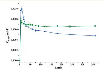
Fig. 13 Dissolution profiles of pure CBZ (■) and CBZ cocrystal (■).
