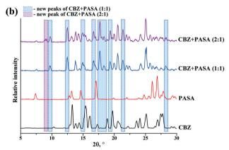
Fig. 2 (a) DSC heating curves and (b) experimental XRPD patterns of pure carbamazepine (black), para-aminosalicylic acid (red), and 1:1 (blue) and 2:1 (purple) mixtures of compounds after cogrinding.
