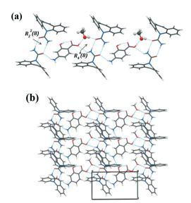
Fig. 8 (a) Layer formed by hydrogen bonded tetramers and (b) packing diagram of [CBZ + PASA + MeOH] (2:1:1).
