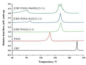
Fig. 11 DSC curves of CBZ, PASA, [CBZ + PASA] (1:1), [CBZ + PASA +  $H_2O$ ] (2:1:1) and [CBZ + PASA + MeOH] (2:1:1) recorded at 10 °C min<sup>-1</sup> heating rate.
