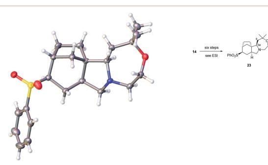
Fig. 3 Crystal structure of 23 with ellipsoids drawn at the 50% probability level. The structure contains one molecule of dichloromethane per molecule of 23 which has been omitted for clarity.
