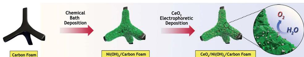
Fig. 1 Process for the design of a self-supported CeO<sub>2</sub>/Ni(OH)<sub>2</sub>/NOSCF electrode and application for the oxygen evolution reaction.
