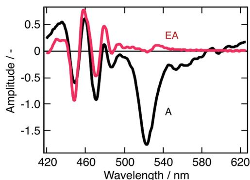
Fig. 5 Modeled electroabsorption signal of a suspension of  $\text{CH}_3\text{NH}_3\text{PbBr}_3$  nanoparticles in chlorobenzene. The blue part of the observed transient absorption spectrum measured at a time delay of 2 ps (black line) fits well with a simulated electroabsorption spectrum (red) dominated by the second derivative component of the ground state absorption spectrum (see ESI† for details).
