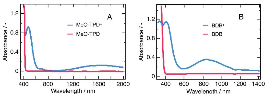
Fig. 7 Absorption spectra of both quenchers in the neutral (red) and oxidized (blue) forms. (A) MeO-TPD and (B) 1,4-bis(diphenylamino)benzene (BDB). The spectra of the oxidized species have been recorded after quantitative reaction of the neutral compounds with the one-electron oxidizer  $\text{NOBF}_4$ .
