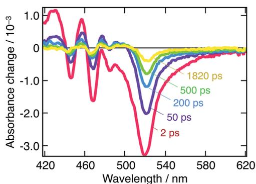
Fig. 2 Transient absorption spectra of a suspension of  $\text{CH}_3\text{NH}_3\text{PbBr}_3$  nanoparticles in chlorobenzene at different time delays following  $\lambda_{\text{ex}} = 390$  nm pulsed excitation. Red:  $t = 2$  ps, purple:  $t = 50$  ps, blue:  $t = 200$  ps, green:  $t = 500$  ps, and yellow:  $t = 1820$  ps.
