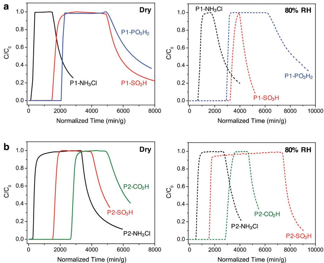
Fig. 3 Ammonia breakthrough curves for (a) P1 and (b) P2 polymers under dry (left, solid lines) and humid (right, dashed lines) conditions at 293 K. The challenge concentration ( $C_0$ ) of ammonia in air was  $2000 \text{ mg m}^{-3}$  with a flow rate of  $20 \text{ mL min}^{-1}$ . Once saturation was achieved, desorption curves were obtained upon purging the column with air under the corresponding initial dry or humid condition.
