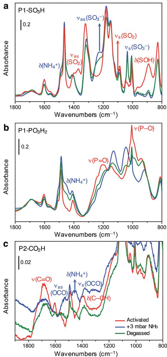
Fig. 4 Infrared spectra of (a) P1-SO<sub>3</sub>H, (b) P1-PO<sub>3</sub>H<sub>2</sub>, and (c) P2-CO<sub>2</sub>H in the 1800–800 cm<sup>-1</sup> spectral range collected at 298 K after its thermal activation under vacuum (red lines), equilibration with ammonia at an equilibrium pressure of 3 mbar (blue lines), and subsequent evacuation under vacuum (green lines).
