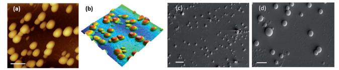
Fig. 2 Microscopy analysis. (a) AFM micrograph of 1 (scale bar = 500 nm). (b) 3D height profile of the spherical structures of 1. (c) SEM micrograph (scale bar =  $2 \mu m$ ). (d) Zoomed view (scale bar =  $1 \mu m$ ).
