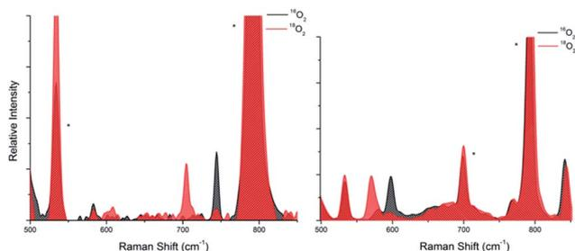
Fig. 3 Resonance Raman spectrum of **P4** (left) in THF and **O7** (right) in THF/pentane (1 : 1) at 193 K. The <sup>16</sup>O<sub>2</sub> spectra are in black and the <sup>18</sup>O<sub>2</sub> spectra are in red. Residual solvent signals are marked with an asterisk (\*).
