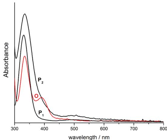
Fig. 5 UV-vis monitoring of the reaction sequence demonstrating the interconversion of P<sub>6</sub> to O<sub>8</sub> using <sup>H,H</sup>BOX as a base and subsequent conversion of O<sub>8</sub> back to P<sub>6</sub> upon addition of [Cu(MeCN)<sub>4</sub>]ClO<sub>4</sub> in the presence of O<sub>2</sub> (baseline correction and dilution factor applied).
