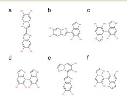
Fig. 5 Molecular structures of 6 structural unique dimers. The most stable dimer is made through (a) 2,2'-position, followed by (b) 2,4'-position (+1.82 kcal mol<sup>-1</sup>), (c) 4,4'-position (+2.19 kcal mol<sup>-1</sup>), (d) 4,7'-position (+2.31 kcal mol<sup>-1</sup>), (e) 2,7'-position (+2.82 kcal mol<sup>-1</sup>), and (f) 7,7'-position (+3.20 kcal mol<sup>-1</sup>).
