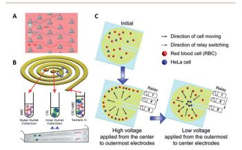
Fig. 3 Device design and working principle of hydrodynamics (A and B) and dielectrophoresis (C) for CTC enrichment. (A) DLD array (modified from ref. 25). (B) Spiral channel with a trapezoidal crosssection (adapted from ref. 27). (C) Dielectrophoresis in a stepping electric field (adapted from ref. 35).
