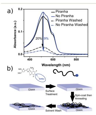
Fig. 3 (a) Thin-film UV-visible spectra of P3OT-PFB modified with 3mercaptopropyl(trimethoxysilane) showing the effect of glass pretreatment, and a subsequent solvent wash (chloroform), on film retention. Films spun from THF solutions (5 mg mL<sup>-1</sup>) (b) schematic representation of partial polymer retention due to tethering to the glass substrate via the siloxane linker (blue dot).
