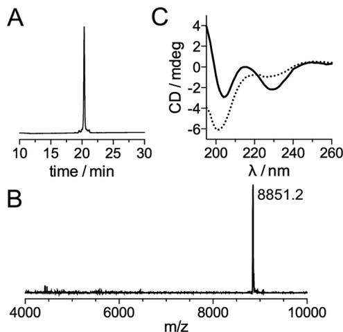
**Fig. 2** (A) HPLC chromatogram and (B) MALDI-TOF spectrum of purified apo-LTIS<sup>Tb</sup> (expected MW = 8850.8). (C) CD spectra of the apo- (dotted line) and Zn-loaded (solid line) forms of LTIS<sup>Tb</sup> (5 μM) recorded in a phosphate buffer (10 mM, pH 7.0).
