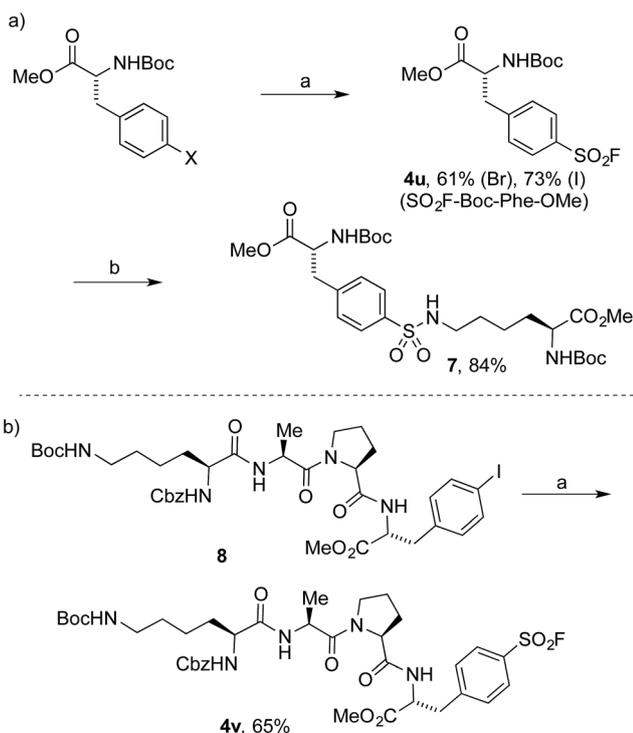
**Scheme 2** Synthesis of amino acid and peptidic sulfonyl fluorides. (a) Reaction conditions: (i) aryl halide (0.4 mmol), PdCl<sub>2</sub>(AmPhos)<sub>2</sub> (5 mol%), DABSO (0.6 equiv.), Et<sub>3</sub>N (3.0 equiv.), *i*-PrOH [0.2 M], 75 °C, 16 h. (ii) NFSI (1.5 equiv.), rt, 3 h. (b) *N*-Boc-L-Lys-OMe, *i*-Pr<sub>2</sub>NEt, DMSO, 100 °C, 15 h. Isolated yields.
