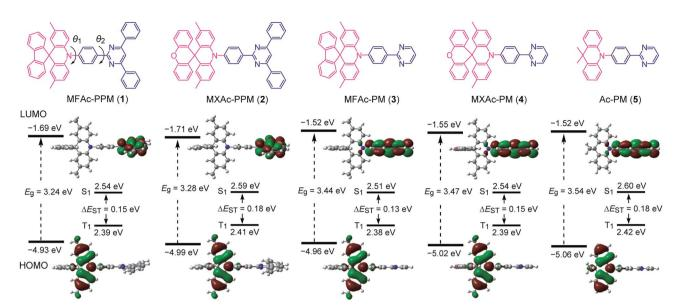
Fig. 2 Chemical structures (upper), HOMO and LUMO distributions, and calculated singlet (S1) and triplet (T1) energy levels (lower) for D-A molecules 1-5 characterized using TD-DFT at the PBE1PBE/6-31G(d) level.
