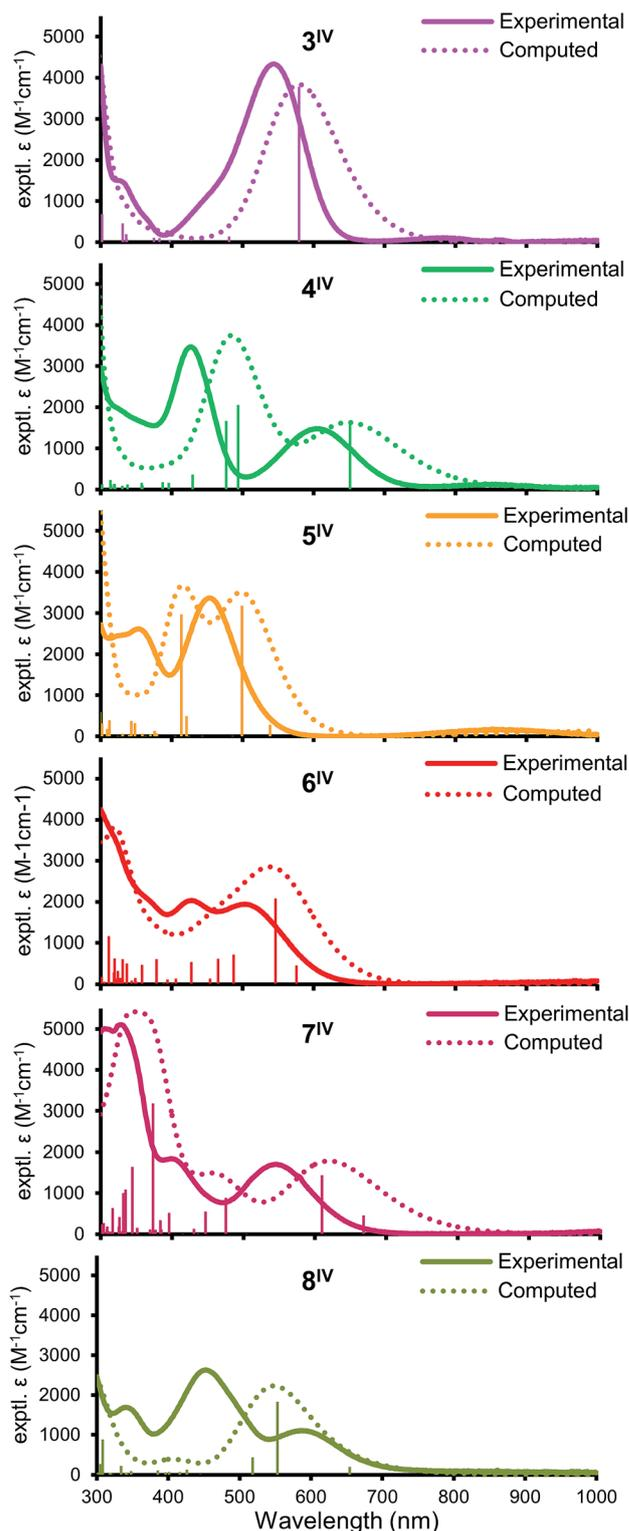
Fig. 3 Experimental UV-visible spectra (solid), along with DFT-computed spectra (dotted) and corresponding excitations (vertical lines) for **3<sup>IV</sup>–8<sup>IV</sup>** in dichloromethane (1 : 1 ethyl acetate/dichloromethane for **8<sup>IV</sup>**). Absolute DFT intensities are arbitrarily scaled.
