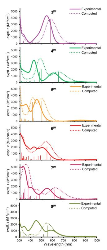
Fig. 3 Experimental UV-visible spectra (solid), along with DFT-computed spectra (dotted) and corresponding excitations (vertical lines) for  $\mathbf{3^{IV}} - \mathbf{8^{IV}}$  in dichloromethane (1:1 ethyl acetate/dichloromethane for  $\mathbf{8^{IV}}$ ). Absolute DFT intensities are arbitrarily scaled.
