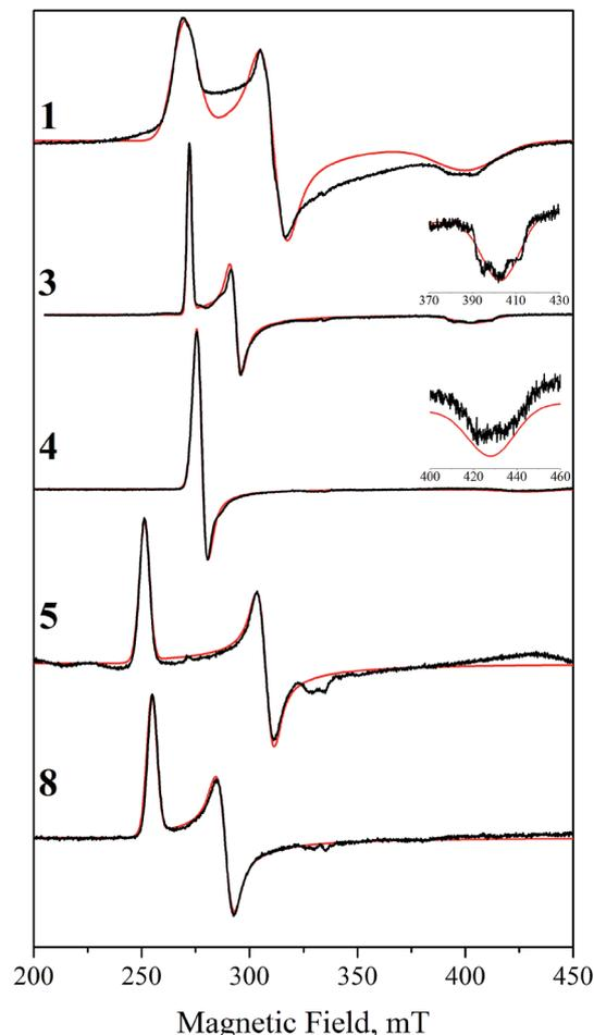
**Fig. 4** X-band EPR spectra for Ir(IV) species in glassed frozen solutions (black) and corresponding simulated spectra (red). Inserts are provided for the high-field peaks of 3 and 4. Note that features near 330 mT are due to trace Cu(II) contamination.
