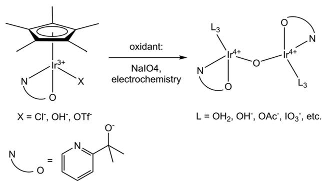
Scheme 1 Transformation of organometallic precursors to highly active water-oxidation catalysts. Proposed catalyst resting state shown on right, accounting for current structural uncertainty.<sup>5</sup>
