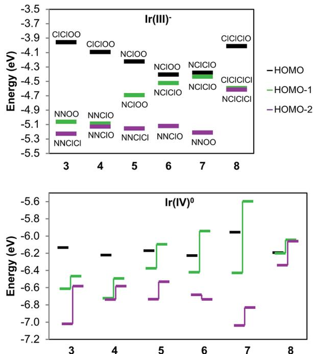
Fig. 5 Computed energies for the three frontier occupied electronic levels (Ir-centered  $t_{2g}$  orbitals) of **3–8** in each oxidation state, labeled with their corresponding coplanar ligands (same legend and labeling applies to both graphs). Bottom: alpha and beta spin levels correspond to leftward and rightward bars, respectively; paired levels are connected by vertical lines and color (the virtual beta SOMO is not shown).
