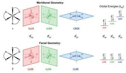
Fig. 1 Effect of ligand arrangement (isomerism) on valence electron energies for the  $d_{\pi}$  orbitals of a  $[ML_3X_3]$ -type  $d^6$  low-spin octahedral complex. In this example, ligand X has a higher donor strength than L. The unequal ligand field exerted on the orbitals of the meridional isomer (such as complex 1) results in a higher HOMO energy than for the facial one (complex 2), thus lowering the energy needed for one-electron oxidation.
