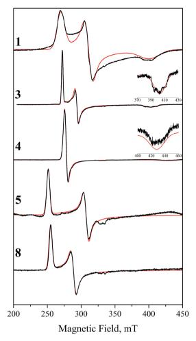
Fig. 4 X-band EPR spectra for Ir(v) species in glassed frozen solutions (black) and corresponding simulated spectra (red). Inserts are provided for the high-field peaks of **3** and **4**. Note that features near 330 mT are due to trace Cu(u) contamination.
