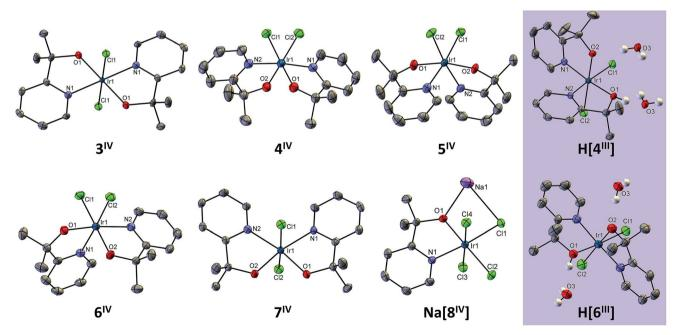
Fig. 2 ORTEP crystal structures of  $3-8^{IV}$  and  $4^{III}$  and  $6^{III}$  drawn at the 50% probability level. Solvent molecules are omitted for clarity, except for the water molecules in the Ir(III) structures. Hydrogen atoms are similarly omitted, except at alkoxo positions (all alkoxos are deprotonated unless explicitly drawn). Drawings of  $4^{III}$  and  $6^{III}$  both show one of two disordered states, the other having a proton at O2 instead of O1.
