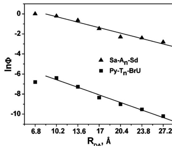
Fig. 5 The distance dependence of the generation yield of the reduced product. The hole transport yield in Sa–A<sub>n</sub>–Sd was also plotted. Reprinted with permission from literature.<sup>47</sup> Copyright (2009) American Chemical Society.
