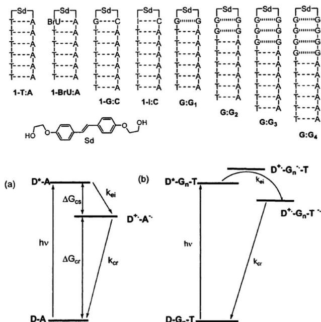
Fig. 4 DNA hairpins conjugated with Sd at the loop position and schematic energy diagram for the excess electron injection from the photoexcited Sd. Reprinted with permission from literature.<sup>46</sup> Copyright (2002) American Chemical Society.
