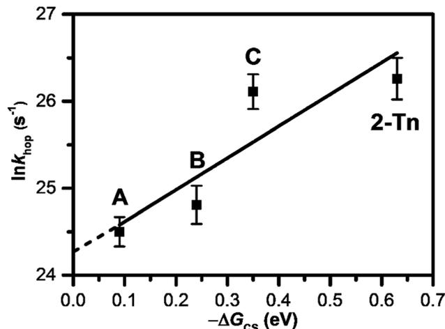
Fig. 9 Dependence of  $\ln k_{\text{hop}}$  on  $-\Delta G_{\text{CS}}$ . A, B, C, and 2-Tn were estimated from DNA conjugated with 4T, <sup>A</sup>Py', 3E, and 2E, respectively, as a photosensitizing electron donor. Reprinted with permission from literature.<sup>61</sup> Copyright (2016) American Chemical Society.
