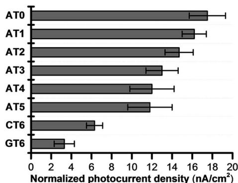
Fig. 14 Normalized photocurrent density of DNA-modified electrode. Error bars represent the standard deviation from five experiments. Reprinted with permission from literature.<sup>77</sup> Copyright (2016) John Wiley and Sons.
