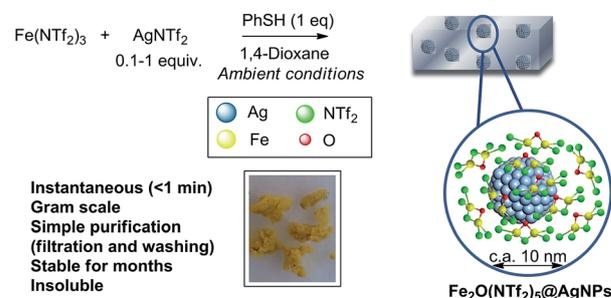
Fig. 1 Synthesis of Fe<sub>2</sub>O(NTf<sub>2</sub>)<sub>5</sub>@AgNPs. Reaction conditions: Fe(NTf<sub>2</sub>)<sub>3</sub> (6.16 mmol), AgNTf<sub>2</sub> (0.1–1.0 equivalent), thiophenol (6.16 mmol), 1,4-dioxane (80 mL), room temperature, <1 min to 1 h, 28–90% yield. See details in ESI.† A photograph of the yellow solid and a model (not scaled) are also provided.
