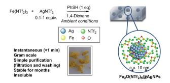
Fig. 1 Synthesis of Fe $_2$ O(NTf $_2$ ) $_5$ @AgNPs. Reaction conditions: Fe (NTf $_2$ ) $_3$  (6.16 mmol), AgNTf $_2$  (0.1–1.0 equivalent), thiophenol (6.16 mmol), 1,4-dioxane (80 mL), room temperature, <1 min to 1 h, 28–90% yield. See details in ESI.† A photograph of the yellow solid and a model (not scaled) are also provided.
