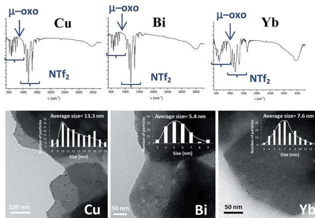
Fig. 10 Top: FT-IR spectra of the solids made by the same procedure as  $\text{Fe}_2\text{O}(\text{NTf}_2)_5@Ag\text{NPs}$  but with  $\text{Cu}(\text{NTf}_2)_2$ ,  $\text{Bi}(\text{NTf}_2)_3$  and  $\text{Yb}(\text{NTf}_2)_3$  as starting materials, from left to right, respectively. Bottom: transmission electron microscopy (TEM) photographs with the corresponding histograms for, at least, 5 different photos.
