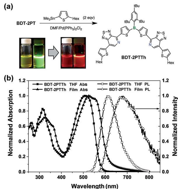
Fig. 9 (a) Synthesis of **BDT-2PTTh** (Hex = *n*-hexyl) and corresponding photographs of DCM solutions under natural light and upon irradiation with a UV lamp (365 nm); (b) UV-Vis and photoluminescence spectra of **BDT-2PTTh** in THF and as thin film.
