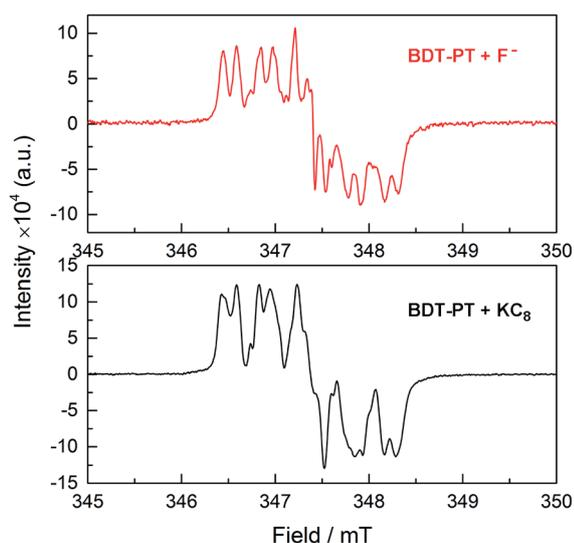
Fig. 8 (Top) EPR data after addition of TBAF·3H<sub>2</sub>O to a solution of **BDT-PT** in THF; (bottom) EPR data after addition of a small amount of K<sub>2</sub>C<sub>8</sub> to a solution of **BDT-PT** in THF.
