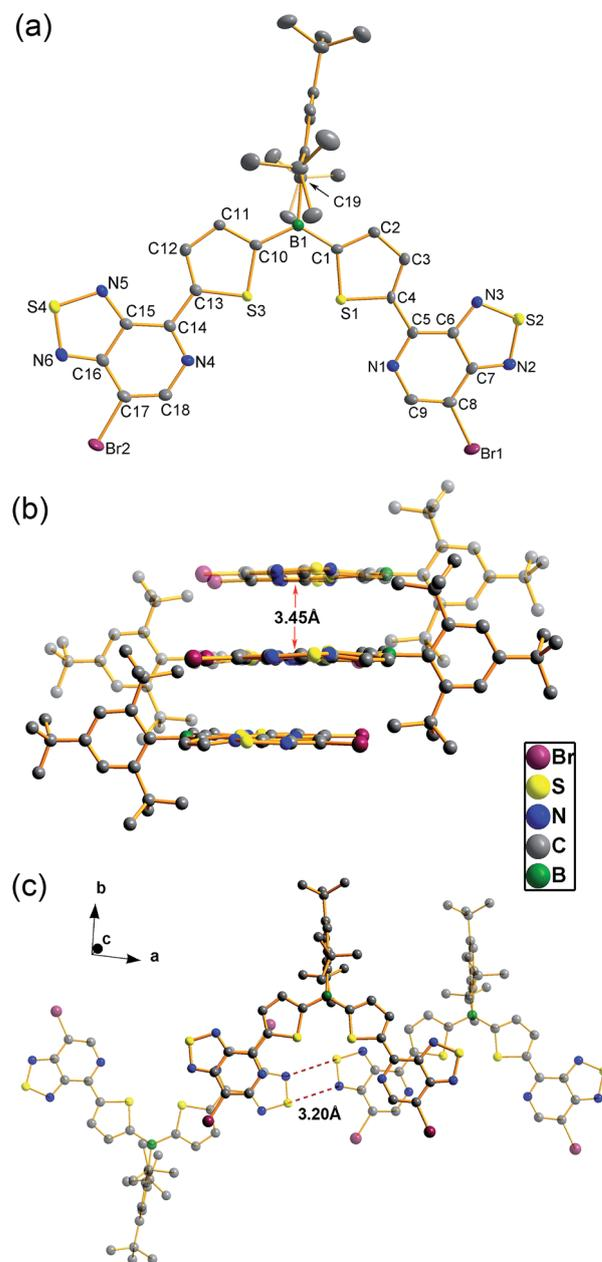
Fig. 1 (a) ORTEP plot of the single crystal X-ray structure of **BDT-2PT** (30% thermal ellipsoids, cocrystallized THF molecule and H atoms are omitted); (b) illustration of  $\pi$ -stacking along the crystallographic *c*-axis; (c) illustration of intra-layer interactions.
