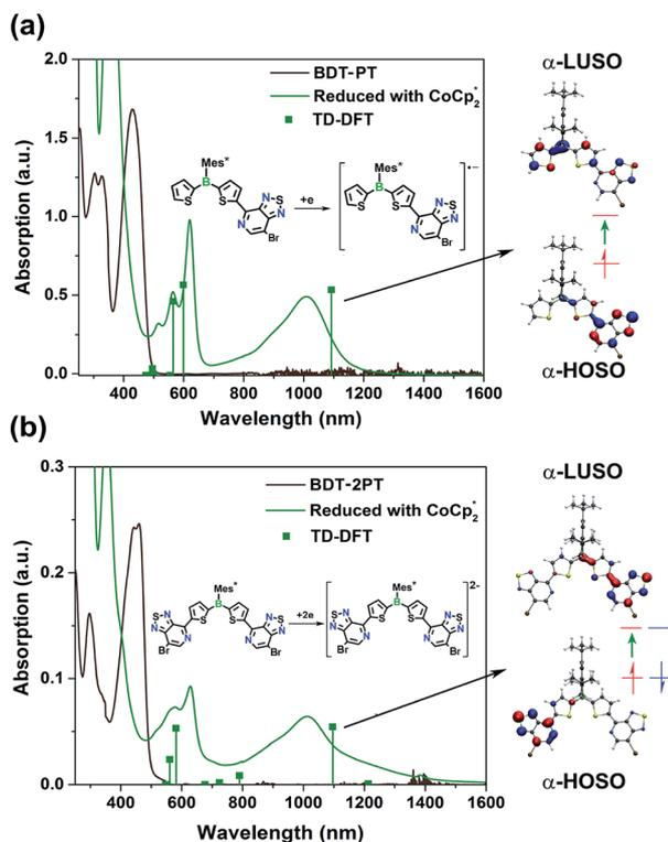
Fig. 5 UV-Vis spectra of (a) BDT-PT and (b) BDT-2PT before (black) and after (green) chemical reduction with  $\text{Cp}_2\text{Co}$  in THF. Droplines with squares correspond to the TD-DFT results for the radical anion/dianion. Right: Illustration of electronic transitions of  $\text{BDT-PT}^{\bullet-}$  and  $\text{BDT-2PT}^{2-}$  corresponding to the lowest energy absorptions at *ca.* 1000 nm. Peaks at  $<400$  nm are due to excess  $\text{Cp}_2\text{Co}$ .
