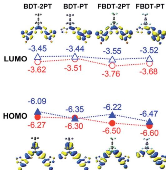
Fig. 4 HOMO and LUMO orbitals of borane-PT dyads and triads (structures optimized at B3LYP/6-31+G\* level, single point energy calculations at B3PW91/6-311+G\*\*). Red circles correspond to DFT results, blue triangles to experimental results using  $E_{\text{LUMO}} = -4.8 - E_{\text{red}}$  (eV),  $E_{\text{gap}} = 1240/\lambda_{\text{onset}}$  (eV).
