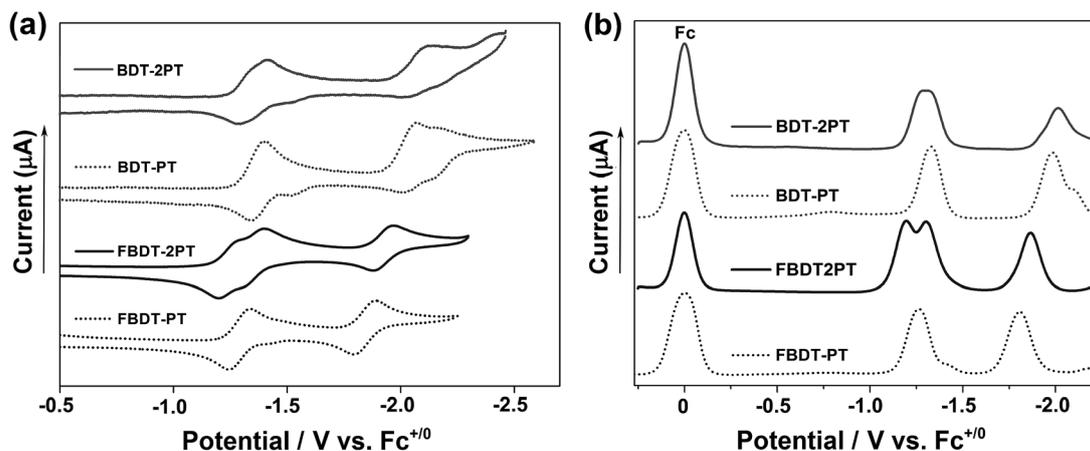
Fig. 3 (a) Cyclic voltammetry (CV) and (b) square wave voltammetry (SWV) data in THF/0.1 M  $\text{Bu}_4\text{N}[\text{PF}_6]$  ( $1 \times 10^{-3}$  mol  $\text{L}^{-1}$ ; vs.  $\text{Fc}^{0/+}$ ,  $\nu = 100$  mV  $\text{s}^{-1}$ ).
