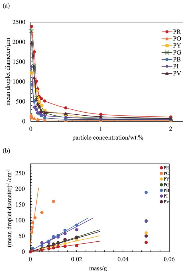
Fig. 9 (a) Variation of the mean droplet diameter after 3 months with particle concentration for the seven pigment-stabilised emulsions,  $\phi_w = 0.5$ , (b) plot of inverse of mean droplet diameter against initial mass of particles for emulsions in (a).
