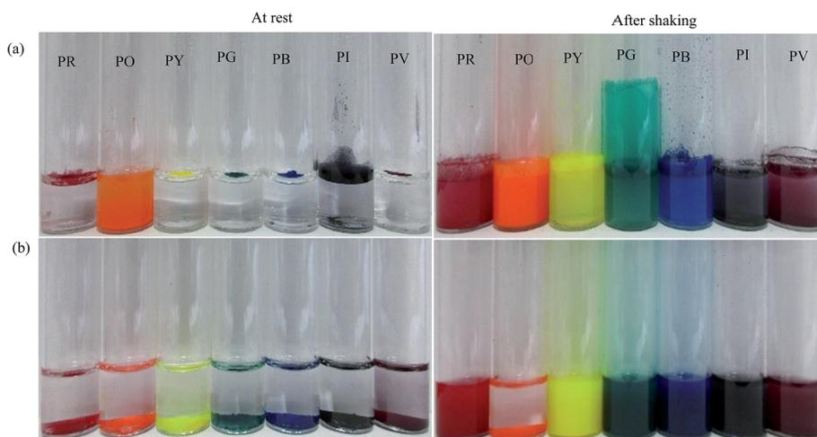
**Fig. 4** Photos of vessels showing the appearance of a mixture of 50 mg of pigment particles and  $3 \text{ cm}^3$  of either (a) water or (b) *n*-heptane before and after agitation for 30 s.
