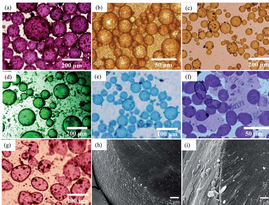
Fig. 8 Optical microscope images of emulsions taken after 20 min for  $\phi_w = 0.5$  prepared at 1 wt% particles and the seven pigments for (a) PR, (b) PO, (c) PY, (d) PG, (e) PB, (f) PI, (g) PV. Emulsions are w/o except those of PO which are o/w. Cryo-SEM images for emulsions of (h) PY and (i) PR.
