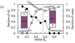
Fig. 12 Variation of fraction of oil (filled points) and water (open points) resolved after two months as a function of initial water volume fraction for emulsions in Fig. 10 for (a) PO, (b) PG, (c) PV.
