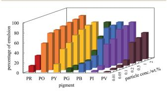
Fig. 6 Percentage of emulsion remaining after three months for the seven pigments at various particle concentrations for  $\phi_{\rm w}=0.5$ . Emulsions are w/o except those of PO which are o/w.
