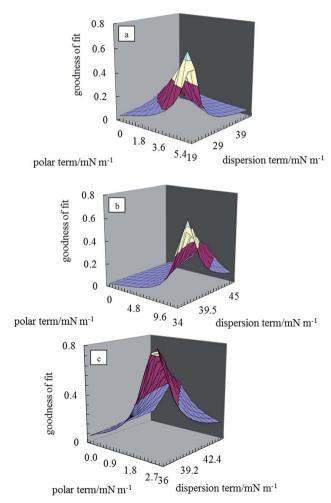
Fig. 2 3-D surface energy plots for disks of the pigment particles for different values of  $\gamma_{\rm sa}^{\rm d}$  and  $\gamma_{\rm sa}^{\rm p}$  for pigments (a) PR, (b) PO, (c) PV.
