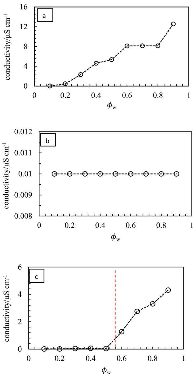
Fig. 11 Variation of emulsion conductivity as a function of  $\phi_w$  for the emulsions in Fig. 10 for (a) PO – o/w, (b) PG – w/o, (c) PV – w/o to o/w. The vertical dotted line signifies catastrophic phase inversion.
