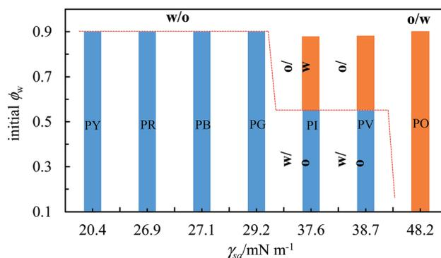
Fig. 15 Correlation between transitional phase inversion (induced by a change in particle surface energy) and catastrophic phase inversion (induced by a change in  $\phi_w$ ) of heptane-water emulsions stabilized by pigment particles of different type.
