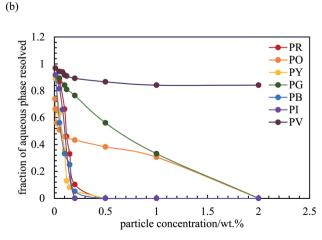
Fig. 7 Fraction of (a) oil and (b) aqueous phase resolved after three months from emulsions stabilized by the seven pigments,  $\phi_{\rm w}=0.5$ , as a function of particle concentration.
