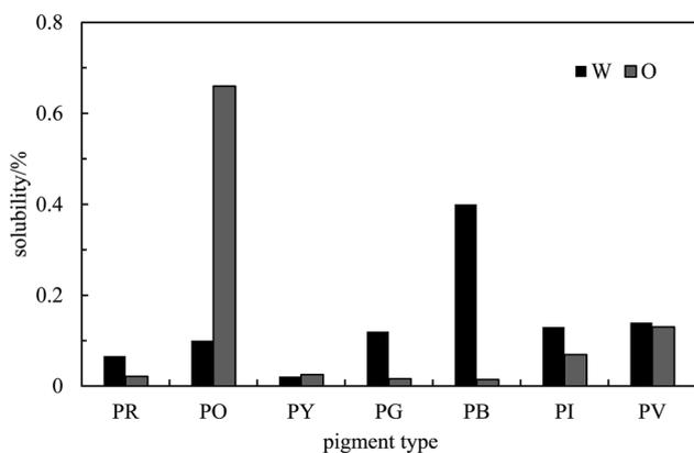
**Fig. 3** Solubility of the seven pigments in water (W) and *n*-heptane (O) determined by spectrophotometry at room temperature.
