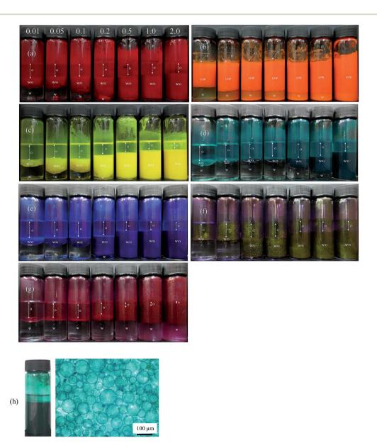
Fig. 5 Photographs of emulsions after 1 month prepared at different particle concentrations (given in wt%) for the seven pigments with  $\phi_{\rm w}=0.5$ : (a) PR, (b) PO, (c) PY, (d) PG, (e) PB, (f) PI, (g) PV. Emulsions are w/o except those of PO which are o/w. In (h), w/o emulsion and microscope image of the mixture containing 0.5 wt% each of PY and PB.
