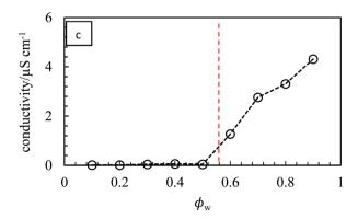
Fig. 11 Variation of emulsion conductivity as a function of  $\phi_{\rm w}$  for the emulsions in Fig. 10 for (a) PO – o/w, (b) PG – w/o, (c) PV – w/o to o/w. The vertical dotted line signifies catastrophic phase inversion.
