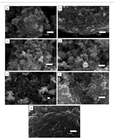
Fig. 1 SEM images of powders of the seven pigments showing the primary particles: (a) PR, (b) PO, (c) PY, (d) PG, (e) PB, (f) PI, (g) PV.
