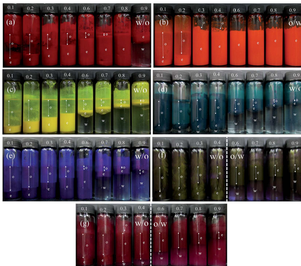
Fig. 10 Photos of vessels after 30 min containing emulsions stabilized by 1 wt% of pigment particles at different values of \phi_w (given) for (a) PR, (b) PO, (c) PY, (d) PG, (e) PB, (f) PI, (g) PV. The dotted line in (f) and (g) signifies catastrophic phase inversion.
