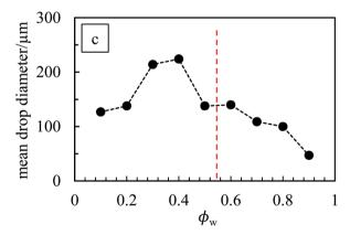
Fig. 14 Variation of average drop diameter with  $\phi_{w}$  for emulsions in Fig. 10 for (a) PO, (b) PG, (c) PV.
