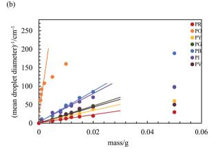
Fig. 9 (a) Variation of the mean droplet diameter after 3 months with particle concentration for the seven pigment-stabilized emulsions,  $\phi_{\rm w}=0.5$ , (b) plot of inverse of mean droplet diameter against initial mass of particles for emulsions in (a).
