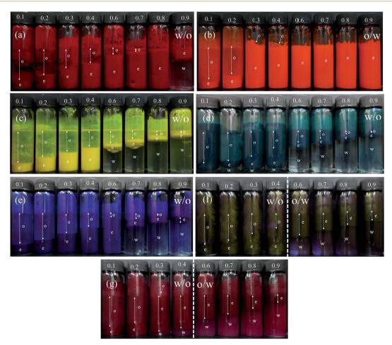
Fig. 10 Photos of vessels after 30 min containing emulsions stabilized by 1 wt% of pigment particles at different values of  $\phi_w$  (given) for (a) PR, (b) PO, (c) PY, (d) PG, (e) PB, (f) PI, (g) PV. The dotted line in (f) and (g) signifies catastrophic phase inversion.
