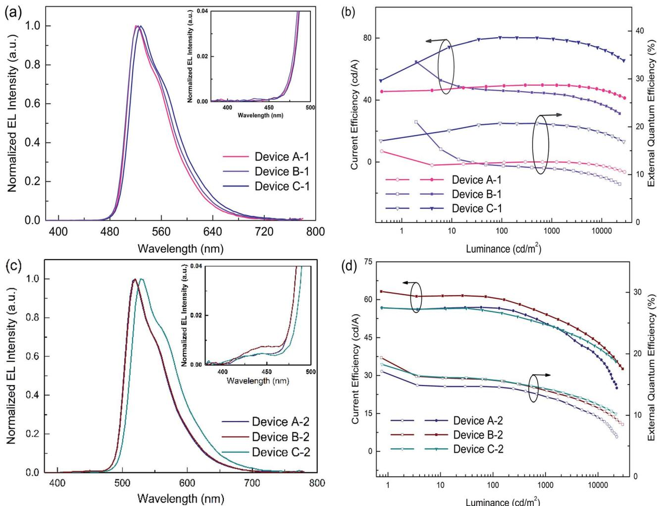
Fig. 4 (a) EL spectra under a luminance of  $1000 \text{ cd m}^{-2}$  and (b) Ce-L-EQE characteristics of devices A-1, B-1 and C-1. (c) EL spectra under the luminance of  $1000 \text{ cd m}^{-2}$  and (d) Ce-L-EQE characteristics of devices A-2, B-2 and C-2. Inset of (a) and (c) shows magnified band edge between 380 and 500 nm.
