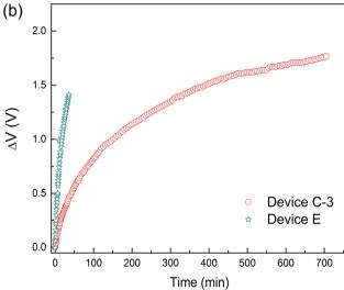
**Fig. 6** Time evolution of the normalized luminance, L, of devices C-3 and E in a dry-nitrogen (<1 ppm  $H_2O$  and  $O_2$ ) atmosphere (a) and change in operating voltage  $\Delta V$  (offset to zero) at the initial luminance of  $L_0=5000$  cd m<sup>-2</sup> (b). The inset of (a) shows the photos of the test device C-3 after 200 min.
