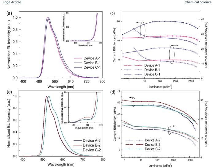
Fig. 4 (a) EL spectra under a luminance of  $1000 \text{ cd m}^{-2}$  and (b) Ce-L-EQE characteristics of devices A-1, B-1 and C-1. (c) EL spectra under the luminance of 1000 cd  $m^{-2}$  and (d) Ce-L-EQE characteristics of devices A-2, B-2 and C-2. Inset of (a and c) shows magnified band edge between 380 and 500 nm
