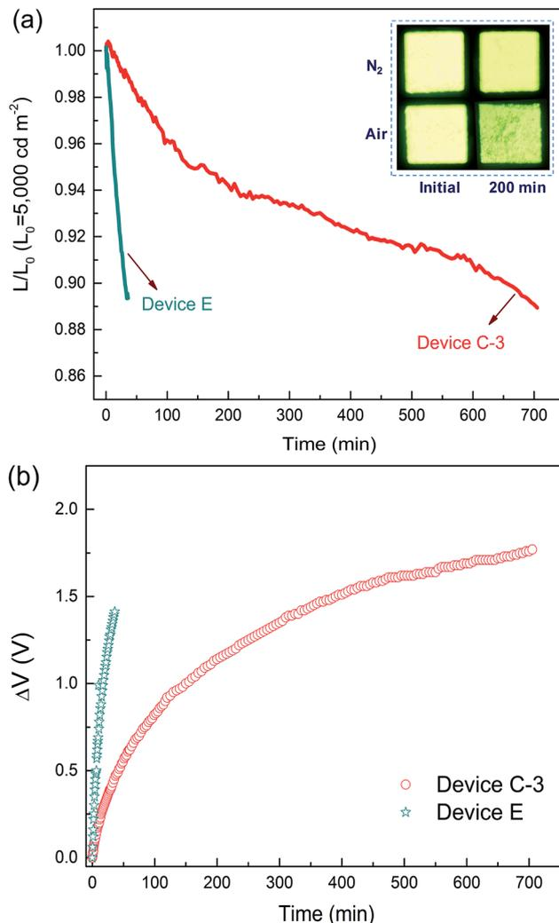
Fig. 6 Time evolution of the normalized luminance,  $L$ , of devices C-3 and E in a dry-nitrogen (<1 ppm H<sub>2</sub>O and O<sub>2</sub>) atmosphere (a) and change in operating voltage  $\Delta V$  (offset to zero) at the initial luminance of  $L_0 = 5000$  cd m<sup>-2</sup> (b). The inset of (a) shows the photos of the test device C-3 after 200 min.
