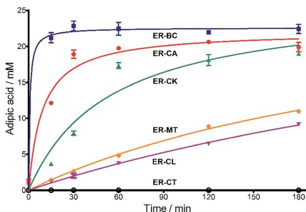
Fig. 1 Time course for the biotransformation of 2-hexenedioic acid into adipic acid by *E. coli* cells expressing ERs. A mixture of *cis*- and *trans*-isomers of 2-hexenedioic acid (20 mM) was used as a substrate. The formation of adipic acid was analyzed using HPLC. (■) = ER-BC, (●) = ER-CA, (▲) = ER-CK, (◆) = ER-MT, (▼) = ER-CL, and (○) = ER-CT.
