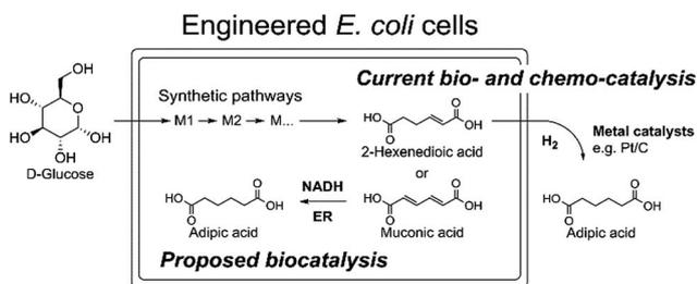
**Scheme 1** The current biocatalytic synthesis of adipic acid from glucose requires chemical hydrogenation of unsaturated six-carbon dicarboxylic acids *e.g.* *cis,cis*-muconic acid or 2-hexenedioic acid.
