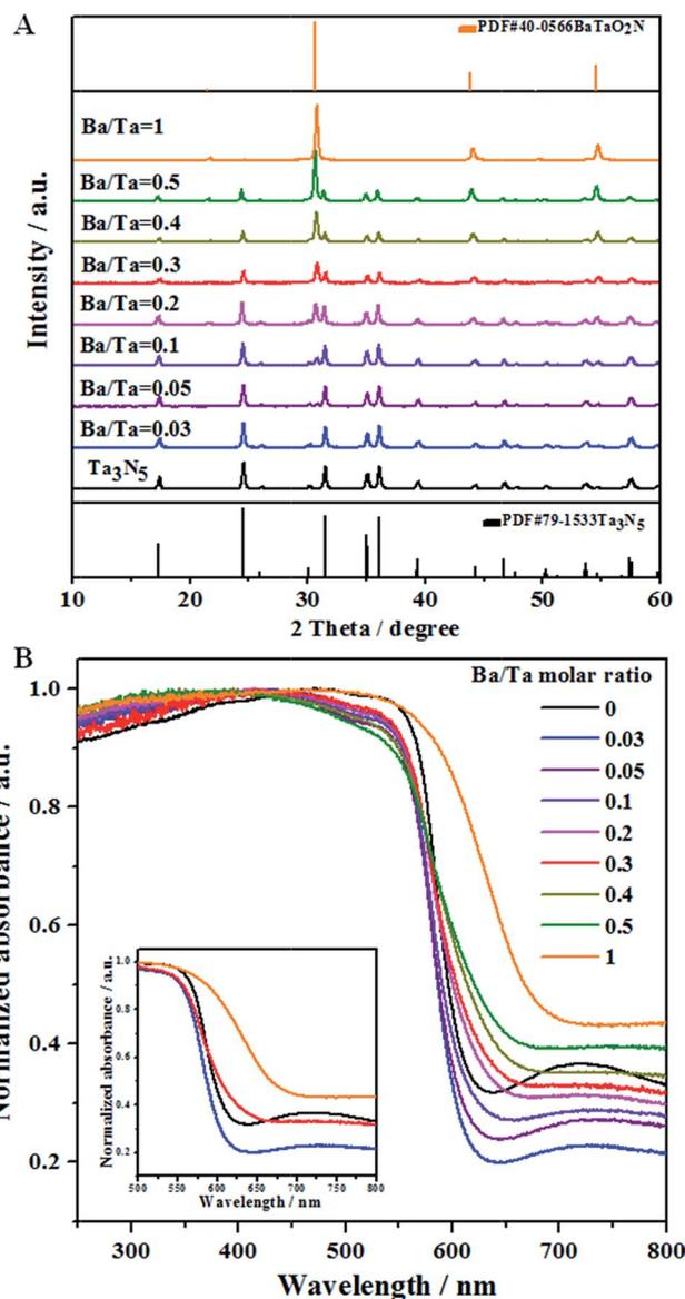
Fig. 1 Structural characterizations of typical  $Ba(n)-Ta_3N_5$  samples ( $n = 0-1$ ): (A) XRD patterns and (B) UV-vis spectra. " $n$ " stands for the molar ratio of Ba/Ta. The inset figure is enlarged for the wavelength range of 500–800 nm.
