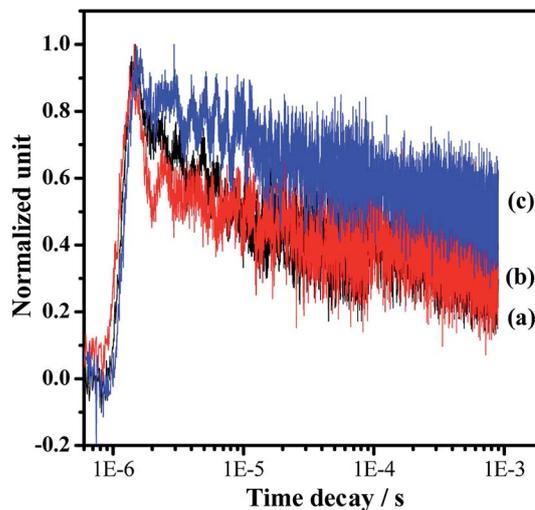
Fig. 6 Normalized transient absorption profiles of the representative samples in a vacuum: (a) Pt/Ta<sub>3</sub>N<sub>5</sub>, (b) Pt/BaTaO<sub>2</sub>N and (c) Pt/Ba(0.3)-Ta<sub>3</sub>N<sub>5</sub>. The pulse laser at 355 nm was used to excite the samples for the IR tests. The cocatalyst of Pt with a loading amount of 0.5 wt% was deposited by impregnation and a subsequent H<sub>2</sub> reduction method.
