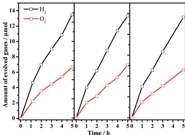
Fig. 5 Multiple cycles of Z-scheme overall water splitting with 0.5 wt% Pt/Ba(0.3)-Ta<sub>3</sub>N<sub>5</sub> and 0.45 wt% PtO<sub>x</sub>/WO<sub>3</sub> as H<sub>2</sub>-evolving and O<sub>2</sub>-evolving photocatalysts, respectively. Reaction conditions: 50 mg of Pt/Ba(0.3)-Ta<sub>3</sub>N<sub>5</sub> and 50 mg of PtO<sub>x</sub>/WO<sub>3</sub>; 100 mL of NaI aqueous solution (1.0 mM); 300 W xenon lamp ( $\lambda > 420$  nm), top-irradiation.
