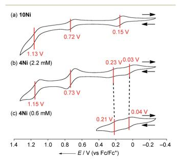
Fig. 5 Cyclic voltammograms of (a) **10N**i, (b) **4N**i at 2.2 mM, and (c) **4N**i at 0.6 mM. The redox potentials were measured by cyclic voltammetry in anhydrous  $CH_2Cl_2$  with 0.1 M  $nBu_4NPF_6$  as a supporting electrolyte, and  $Ag/AgClO_4$  as a reference electrode. The ferrocene/ferrocenium ion couple was used as an external reference. Scan rate: 0.05 V s<sup>-1</sup>.
