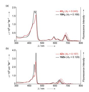
Fig. 1 UV/Vis absorption and emission spectra of (a)  $4H_2$  and  $10H_2$ , and (b) 4Zn and 10Zn in  $CH_2Cl_2$ .  $\varepsilon=$  extinction coefficient.
