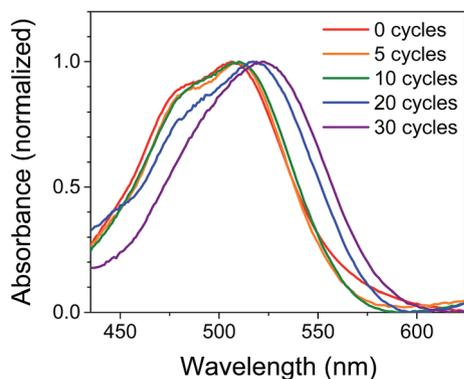
Fig. 2 Normalized UV-Vis absorption spectra of NiO|PMI films treated with 0–30 cycles of Al<sub>2</sub>O<sub>3</sub> ALD. The NiO background is subtracted.
