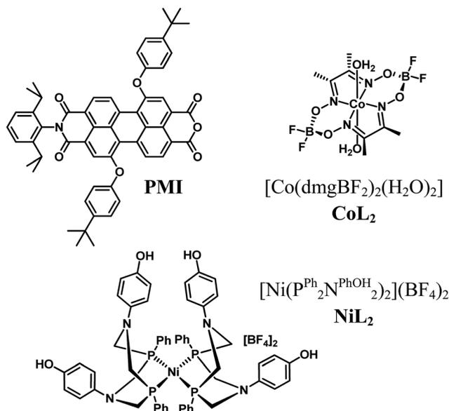
Fig. 1 Chemical structures of the PMI photosensitizer and the H<sub>2</sub> evolution catalysts.
