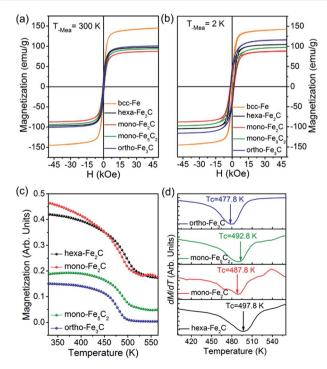
Fig. 7 Magnetic properties of the initial bcc-Fe and the preformed ICNPs. (a and b) M vs. H curves at 300 K and 2 K, respectively. (c and d) M vs. T and the dM/dT curves indicating the Curie temperatures.
