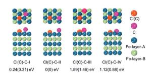
Fig. 6 Top and side views of the adsorption configurations of the second C on the Cl(C) adsorbed Fe (101) surface, and their relative energies with respect to the most stable configuration II – (I) second C on Fe surface hollow-site-A, in which C–Cl(C) distance is 3.07(2.87) Å, (II) second C on Fe surface hollow-site-B, in which C–Cl(C) distance is 3.95(3.94) Å, (III) top-site, and (IV) bridge-site.
