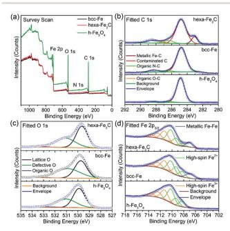
Fig. 2 (a–d) Survey and fitted X-ray photoelectron spectrums (XPS) of hexa-Fe<sub>2</sub>C, bcc-Fe and Fe<sub>3</sub>O<sub>4</sub> NPs. (a) Survey scan. (b) C 1s region. (c) O 1s region and (d) Fe  $2p_{3/2}$  region fitted using Gupta–Sen multiplets.
