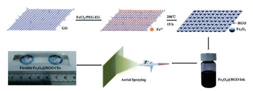
Fig. 30 Schematic diagrams for preparing Fe<sub>3</sub>O<sub>4</sub>@RGO nano-micro composite CEs by a one-pot solvothermal approach and aerial spraying. Reprinted with permission from ref. 564. Copyright (2016) Royal Society of Chemistry.
