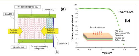
Fig. 13 (a) Bifacial DSSC assembled with a transparent anode and transparent Pt CEs. Reprinted with permission from ref. 205. Copyright (2008) Macmillan Publishers Ltd. (b) Bifacial cells appended with a mirror on the back of CE. Reprinted with permission from ref. 214. Copyright (2017) Elsevier.
