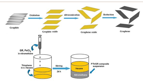
Fig. 22 Fabrication process of the PTh/GR composite. Reprinted with permission from ref. 417. Copyright (2015) Elsevier.
