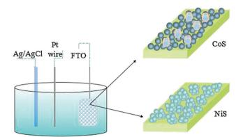
Fig. 27 A diagram of the electrodeposition process of CoS and NiS counter electrodes. Reprinted with permission from ref. 516. Copyright (2015) Elsevier.
