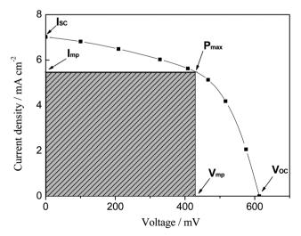
Fig. 9 J-V characteristic curves for the DSSCs
