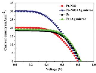
Fig. 29 Photocurrent–voltage (J-V) curves of the DSSCs with Pt–NiO and Pt counter electrodes. Reprinted with permission from ref. 538. Copyright (2015) Springer-Verlag Berlin Heidelberg.
