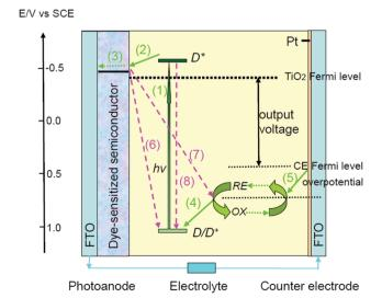
Fig. 5 Fundamental processes and constituent components of dyesensitized solar cells
