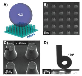
(A) "Fakir"-shaped external side of the PDMS membrane; (B and C) FESEM images of the pillared array uniformly distributed on the PDMS surface; (D) super-hydrophobic nature of the fabricated substrate as verified by water-contact-angle measurements. Reprinted with permission from ref. 195. Copyright (2016) John Wiley & Sons Ltd.
