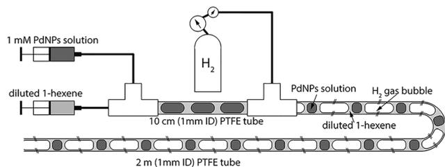
Fig. 4 Schematic of the triphasic segmented flow reactor for hydrogenation reactions to investigate the catalytic activity of PdNPs under minimal mass transfer limitations.<sup>32</sup>
