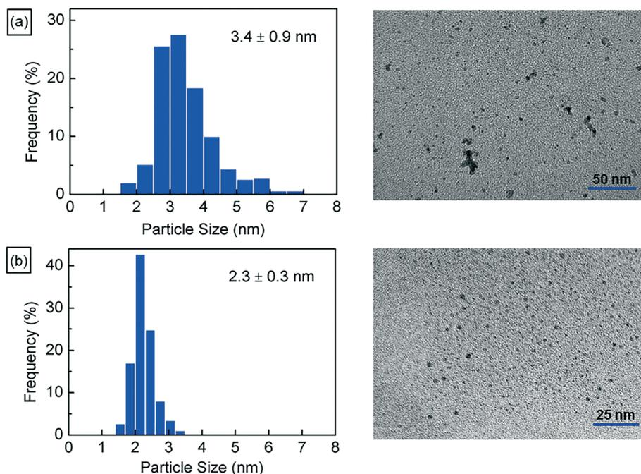
Fig. 3 (a) Particle size distribution and TEM image for batch-synthesized PdNPs with an average size of  $3.4 \pm 0.9$  nm. (b) Particle size distribution and TEM image of flow-synthesized PdNPs with an average size of  $2.3 \pm 0.3$  nm, highlighting smaller mean size and narrower particle size distribution compared to those produced using the small-scale batch reactor.
