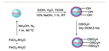
Scheme 1 Schematic diagram for synthesis of Fe<sub>3</sub>O<sub>4</sub>@silica sulfonic acid nanocatalyst
