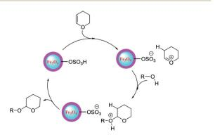
Scheme 3 Proposed mechanism for the tetrahydropyranylation of alcohols using Fe<sub>3</sub>O<sub>4</sub>@SiO<sub>2</sub>@SO<sub>3</sub>H nanocatalyst.
