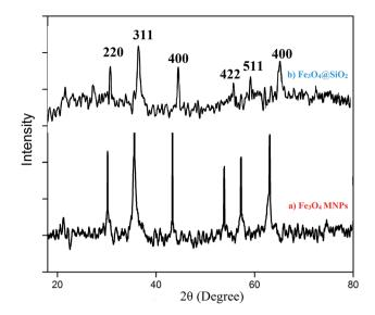
Fig. 2 XRD spectra of (a) Fe<sub>3</sub>O<sub>4</sub>, (b) Fe<sub>3</sub>O<sub>4</sub>@silica sulfonic acid.
