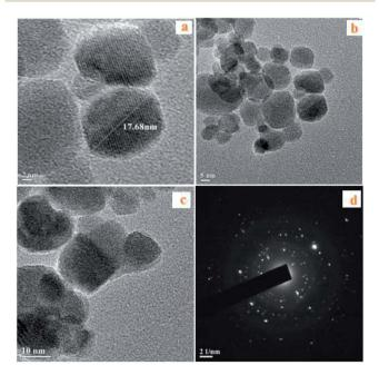
Fig. 3 (a) HRTEM images of  $Fe_3O_4$  nanoparticles, (b) HRTEM images of  $Fe_3O_4$ @SiO<sub>2</sub>, (c) HRTEM images of  $Fe_3O_4$ @SiO<sub>2</sub>@SO<sub>3</sub>H, (d) ED pattern of  $Fe_3O_4$ @SiO<sub>2</sub>@SO<sub>3</sub>H.
