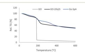
TGA diagrams of derivatives of GO nanoparticles.
