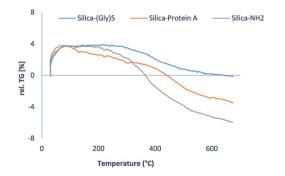
Fig. 3 TG analysis of silica particles after modification
