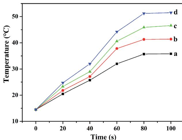
Fig. 4 The microwave thermal response of time-dependent temperature curve for the sodium chloride solution (a), and  $\text{Fe}_3\text{O}_4$  (b), FZAM-APTES (c) and FZA (d) dispersed in sodium chloride solution with microwave irradiation at 2.45 GHz.
