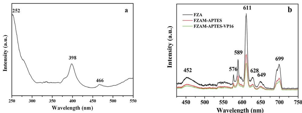
Fig. 3 Excitation spectrum of the FZA nanoparticles at  $\lambda_{\text{em}} = 614 \text{ nm}$  (a); emission spectra of FZA, FZAM-APTES and FZAM-APTES-VP16 nanoparticles at  $\lambda_{\text{ex}} = 398 \text{ nm}$  (b).
