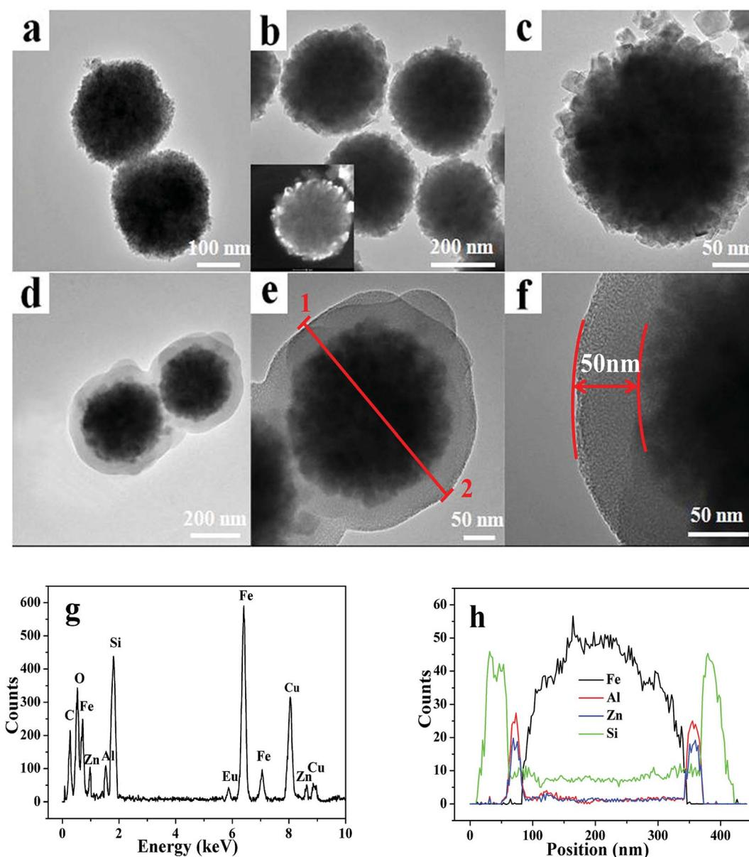
Fig. 2 TEM image of  $\text{Fe}_3\text{O}_4$  (a), FZA (b), HRTEM image of FZA (c), different magnifications of FZAM-APTES microspheres (d-f), energy-dispersive spectrometry (EDS) (g), and line scanning (line 1 and 2) images (h) of FZAM-APTES.
