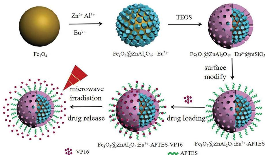
Scheme 1 Schematic illustration of the preparation process of the  $\text{Fe}_3\text{O}_4@\text{ZnAl}_2\text{O}_4:\text{Eu}^{3+}@\text{mSiO}_2\text{-APTES}$  and drug loading and release controlled under microwave irradiation.
