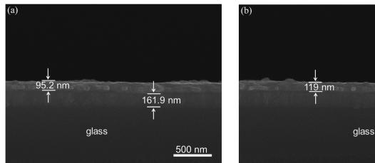
Fig. 2 Cross-section scanning electron microscopic images of the device based on (a) PF-TPA and (b) PF-TPA/MWCNTs composite films.
