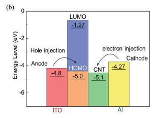
Fig. 8 Energy level diagram of the (a) Al/PF-TPA/ITO and (b) Al/PF-TPA:CNTs/ITO sandwich device.
