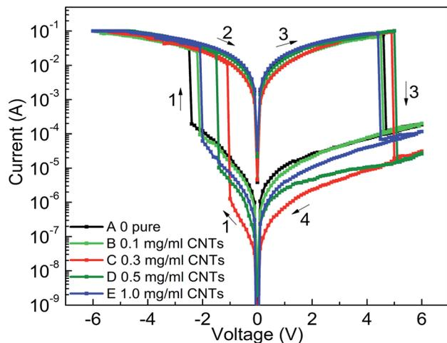
Fig. 4  $I$ - $V$  curves of ITO/PF-TPA:CNTs/Al with different CNTs doping level ( $0 \text{ mg mL}^{-1}$ ,  $0.1 \text{ mg mL}^{-1}$ ,  $0.3 \text{ mg mL}^{-1}$ ,  $0.5 \text{ mg mL}^{-1}$ ,  $1.0 \text{ mg mL}^{-1}$ ).
