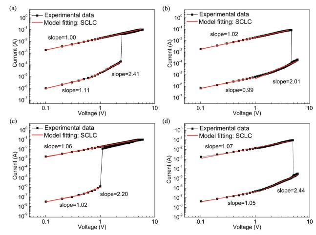
Fig. 7 Linear fitting and corresponding slopes for AI/PF-TPA/ITO (a) set, (b) reset and for AI/PF-TPA:CNTs/ITO device based on sample C. (c) Set, (d) reset.
