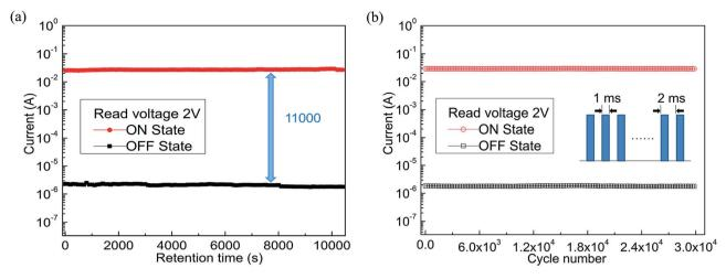
Fig. 6 (a) Retention performance and (b) endurance performance of ITO/PF-TPA:CNTs/Al device on sample C.
