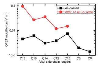
Fig. 9 OFET mobility of Ph- $(Tp)_3$ -Cn before and after TA (TA) at Cr2 phase (all data was obtained from the transfer curves in liner area at  $V_{\rm ds} = -50 \text{ V}$ ).
