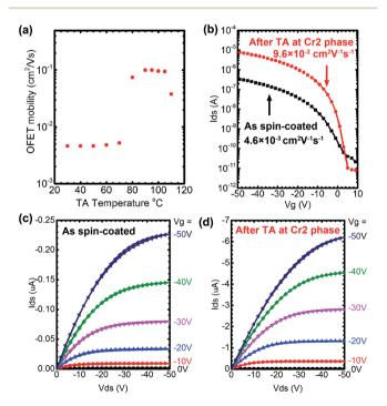
Fig. 8 (a) OFET mobility of Ph-(Tp)<sub>3</sub>-C18 as a function of TA temperatures in the crystal state; (b) typical OFET transfer characteristics of Ph-(Tp)<sub>3</sub>-C18 before and after TA at the Cr2 phase (100 °C); output characteristics of Ph-(Tp)3-C18 (c) as spin-coated, (d) after TA at Cr2 phase (100 °C, 5 min).
