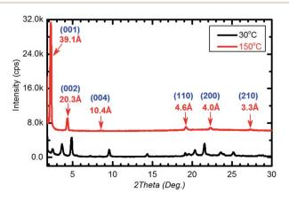
Fig. 4 The bulk film XRD pattern of Ph-(Tp) $_3$ -C18 at different temperatures obtained on heating.
