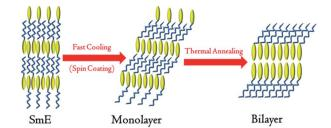
Fig. 7 Schematic of a transition from the SmE phase to a monolayer structure and then a bilayer structure (yellow ellipse represents a rigid core and blue line represents the side alkyl chains).
