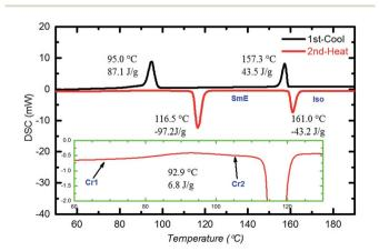
Fig. 2 DSC curves of Ph-(Tp)<sub>3</sub>-C18 at 10 °C min<sup>-1</sup>.
