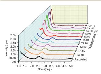
Fig. 6 The thin film XRD pattern of Ph- $(Tp)_3$ -C18 obtained before and after TA at different temperatures in the crystal state (TA at each temperature for 5 min, then cooling to room temperature).
