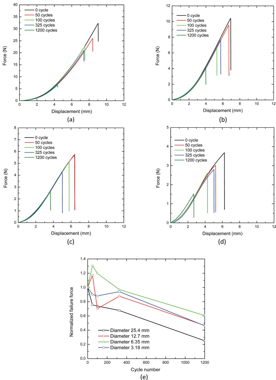
**Fig. 3** Punch test results for separators with different punch size. (a) Punch diameter: 25.4 mm. (b) Punch diameter: 12.7 mm. (c) Punch diameter: 6.4 mm. (d) Punch diameter: 3.175 mm. (e) Normalized failure force vs. cycle number for different punch head sizes.
