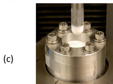
Fig. 1 Volume change of a cycled cell compared with a fresh cell (a) photographs of components of fresh and 1200 cycled lithium ion batteries (b) set-up of separator punch tests with a Teflon punch head of 12.7 mm in diameter (c).
