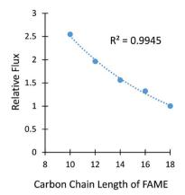
Fig. 5 The relative flux *versus* the number of carbons in FAMEs is shown for a pressure separation using membrane A-2. The line represents an exponential fit.
