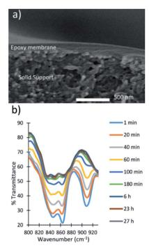
Fig. 4 (a) Cross-sectional image of a spin-coated epoxy membrane. (b) Monitoring the reaction of a spin-coated epoxy membrane *via* FT-IR spectroscopy.
