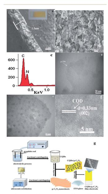
Fig. 2 Cross-section (a) and surface images (b) of the CQD/g-C<sub>3</sub>N<sub>4</sub> film electrode; (c) EDX spectrum of the CQDs/g-C<sub>3</sub>N<sub>4</sub>; (d) TEM image of the  $g-C_3N_4$  nanosheets; (e and f) TEM images of the CQDs/g-C<sub>3</sub>N<sub>4</sub>; and (g) schematic illustration for the preparation of the CQD/g-C<sub>3</sub>N<sub>4</sub> film electrode.
