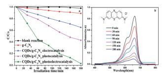
Fig. 9 (a) Different MB degradation processes over the  $g-C_3N_4$  and  $CQD/g-C_3N_4$  photoelectrodes (MB: 5 ppm, 100 mL;  $Na_2SO_4$ : 0.1 M); (b) absorption spectra for the MB solution in the presence of the  $CQD/g-C_3N_4$  photoelectrode under visible light irradiation.
