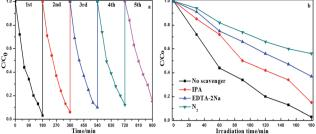
Fig. 12 (a) The recycled 5-CQD/g-C<sub>3</sub>N<sub>4</sub> PEC performance test; and (b) radical trapping experiments during the photocatalytic degradation of MB over the 5-CQD/g-C<sub>3</sub>N<sub>4</sub> composite.
