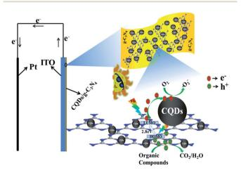
Fig. 16 Mechanism of the photoelectrocatalytic process for the CQDs/g- $C_3N_4$  under visible light irradiation.
