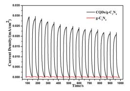
Fig. 14 The transient photocurrent response for g-C<sub>3</sub>N<sub>4</sub> and the CQDs/g-C<sub>3</sub>N<sub>4</sub>.
