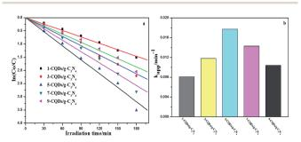
Fig. 10 (a) Photoelectrocatalytic degradation of MB on different electrodes in 0.1 M  $Na_2SO_4$  under visible light irradiation. (b) The corresponding degradation rate constants.
