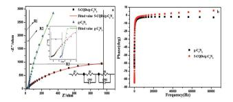
Fig. 15 (a) Electrochemical impedance spectra and (b) the Bode-phase for  $g-C_3N_4$  and the  $5-CQDs/g-C_3N_4$ .
