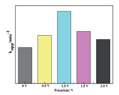
Fig. 11 Photoelectrocatalytic degradation of MB on the 5-CQD/g- $C_3N_4$  electrode at various potentials.
