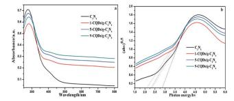
Fig. 4 (a) UV-vis diffuse reflectance spectra of g-C<sub>3</sub>N<sub>4</sub> and the CQD/ g-C<sub>3</sub>N<sub>4</sub> composites with different quantities of the CQDs. (b) The relationship of  $(\alpha h \nu)^{1/2}$  versus photon energy
