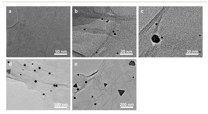
Fig. 3 The real-time TEM images of the as-fabricated nanostructures generated at a desired aging stage. The aging time is 0 minute (a), 30 minutes (b), 60 minutes (c), 12 hours (d), 3 days (e), respectively.
