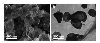
**Fig. 1** The typical SEM (a) and low-resolution TEM (b) images of our Au nanoplates/GO composites.
