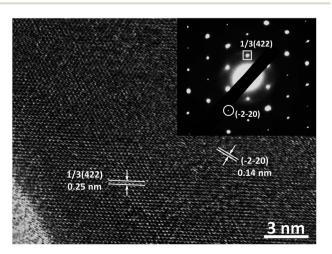
Fig. 4 The typical HRTEM image and the corresponding SAED pattern of our nanoplates obtained with the incident electron beam perpendicular to the basal plane of the nanoplates.
