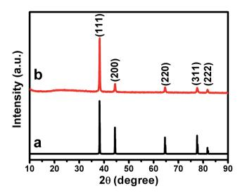
Fig. 5 The XRD pattern of (a) the standard JCPDS file of fcc phase of Au crystal (JCPDS no. 04-0784), and (b) the as-prepared Au nanoplate/GO composites.
