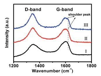
Fig. 7 The typical Raman spectra of our original Au nanoplate/GO composites (I), the used-composites-12 (II), and used-composites-48 (III).
