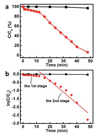
Fig. 6 The catalytic performances (a) and the corresponding kinetic linear simulation curves (b) of our catalysts towards the reduction of 4-NP. Black curves: the results of a blank experiment, wherein no catalysts are used. Red curves: the reaction is conducted in the presence of our Au nanoplates/GO nanocomposites.
