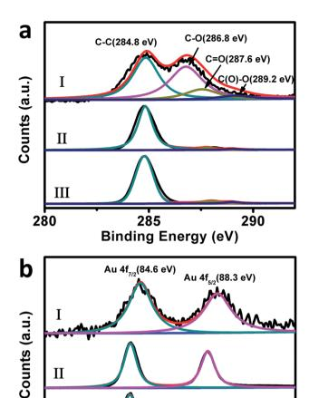
Fig. 8 The C 1s (a) and Au 4f (b) XPS spectra of our original Au nanoplate/GO composites (I), the used-composites-12 (II), and used-composites-48 (III).
