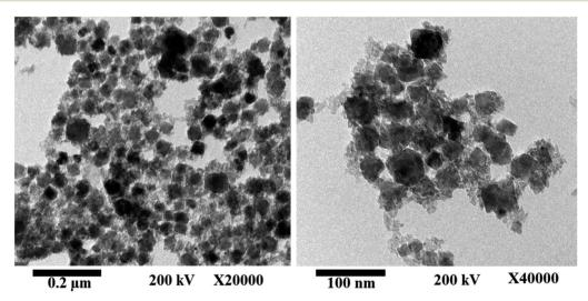
Fig. 2 HR-TEM images of the as-prepared MnCoFeO<sub>4</sub>.
