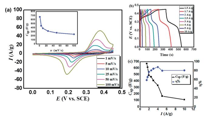
Fig. 4 (a) CV curves recorded for as-prepared MnCoFeO<sub>4</sub> at different scan rates in the potential range of 0-0.45 V<sub>SCE</sub> in the 6 M KOH electrolyte and the inset shows the dependence of the specific capacitance on the scan rate, (b) Galvanostatic charge/discharge curves recorded for MnCoFeO<sub>4</sub>, and (c) the calculated  $C_{sp}$  and  $\eta\%$  at different current densities in the potential range of 0-0.45 V<sub>SCE</sub> in the 6 M KOH electrolyte.
