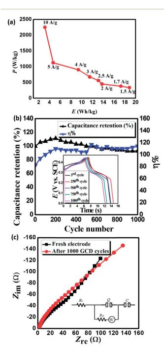
Fig. 5 (a) Ragone plot, (b) cycling stability curves, and (c) Nyquist spectra recorded for MnCoFeO<sub>4</sub> before and after 1000 galvanostatic charge/discharge (GCD) cycles.
