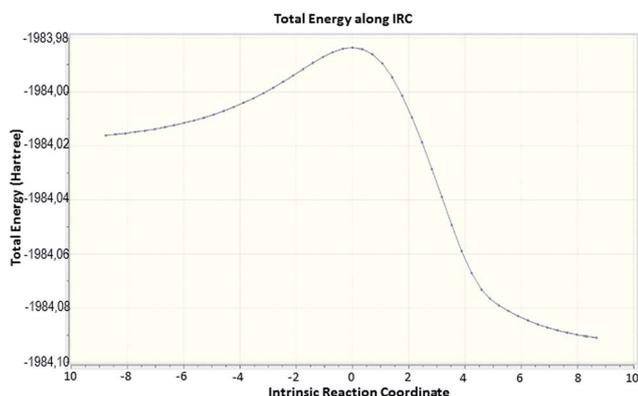
Fig. 4 Reaction energy profile for the cyclization of 21 to 22.
