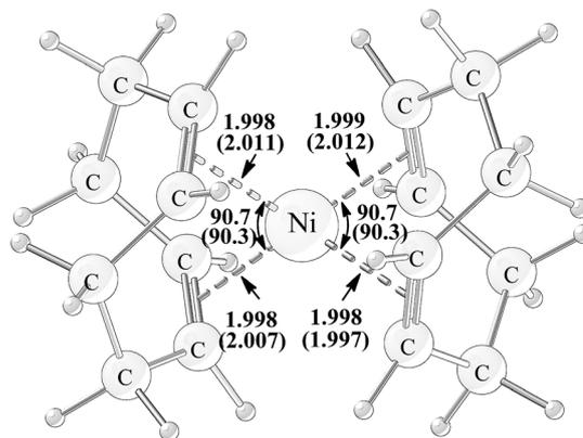
Fig. 1 Geometry structure of Ni(COD)<sub>2</sub> with the calculated and experimentally measured (in parentheses) bond distances (in unit of angstrom) and bite angles (in unit of degree).
