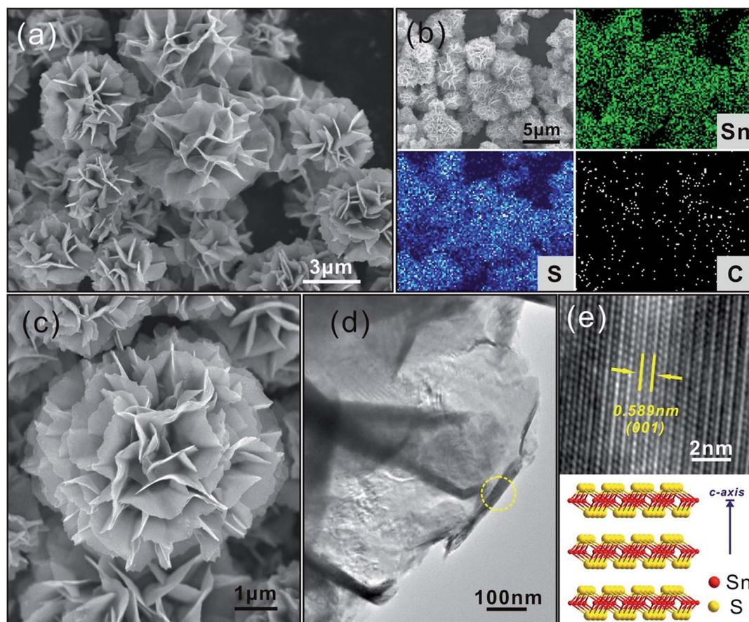
Fig. 5 The morphology and structure of SnS<sub>2</sub>/N-rGO: (a) SEM image of SnS<sub>2</sub>/N-rGO, (b) EDS mapping for each element, (c) the enlarged SEM image of the flower-like SnS<sub>2</sub>/N-rGO composite, (d) TEM image of the SnS<sub>2</sub>/N-rGO sheets and (e) the HRTEM image of the selected area shown in (d), and a schematic of the molecular structure of SnS<sub>2</sub>.
