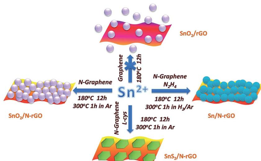
Fig. 2 A schematic of the synthetic routes used to prepare the Sn-based materials supported on rGO and N-rGO.
