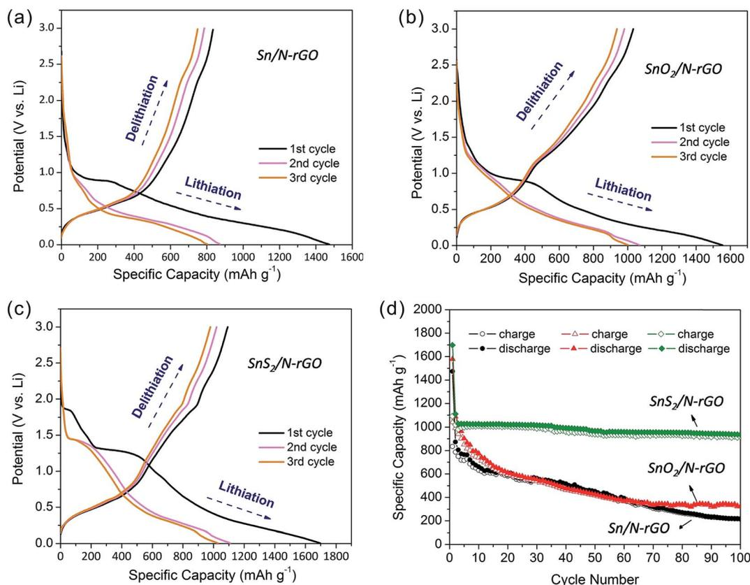
Fig. 6 The galvanostatic charge and discharge curves obtained for the (a) Sn/N-rGO, (b) SnO<sub>2</sub>/N-rGO, and (c) SnS<sub>2</sub>/N-rGO nanocomposites, and (d) their cycling behaviors at a current density of 100 mA h g<sup>-1</sup>.
