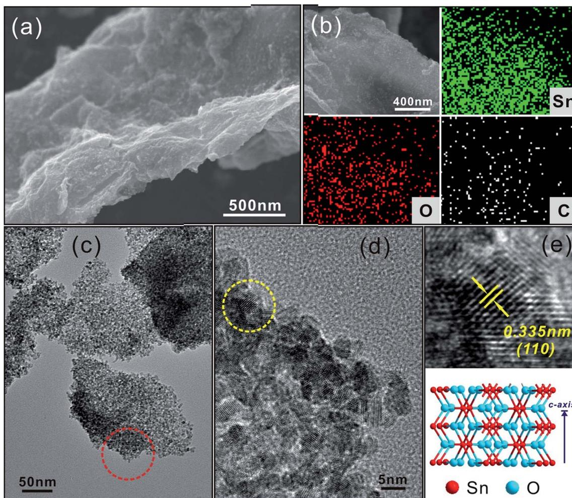
Fig. 3 The morphology and structure of  $\text{SnO}_2/\text{N-rGO}$ : (a) SEM image of  $\text{SnO}_2/\text{N-rGO}$ , (b) EDS mapping for each element, (c) TEM image of the  $\text{SnO}_2/\text{N-rGO}$  composite, (d) the magnified area shown in (c), (e) the HRTEM image of the selected area shown in (d), and a schematic of the molecular structure of  $\text{SnO}_2$ .
