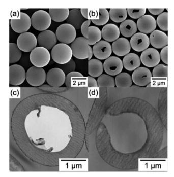
Fig. 2 SEM images (a) and (b) of PS/PDVB particles and TEM images (c) and (d) of ultrathin cross-sections of PS/PDVB particles prepared by seeded polymerizations in the absence (a) and (c) and presence (b) and (d) of SDS. Reproduced from ref. 57 with permission from the American Chemical Society.
