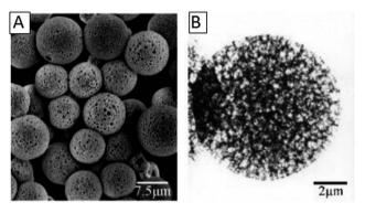
Fig. 4 SEM (A) and TEM (B) images of the hollow core/porous shell of PVAc. Reproduced from ref. 73 with permission from John Wiley and
