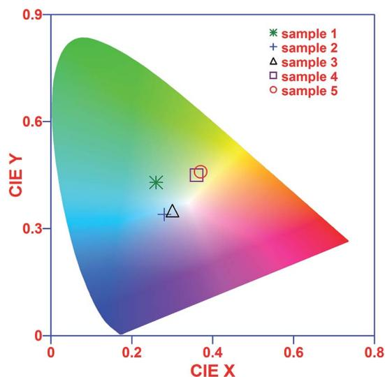
Fig. 9 CIE colour chromaticity diagram of sample 1 (pure  $\gamma\text{-Ga}_{2.67}\text{O}_4$ ), sample 2 ( $\gamma\text{-Ga}_{2.67}\text{O}_4 : 5\text{Sm}$ ), sample 3 ( $\gamma\text{-Ga}_{2.67}\text{O}_4 : 10\text{Sm}$ ), sample 4 ( $\text{Ga}_2\text{O}_3\text{-600}$ ) and sample 5 ( $\text{Ga}_2\text{O}_3\text{-900}$ ).
