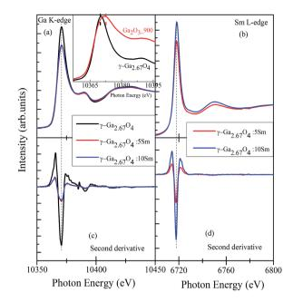
Fig. 4 (a) and (b) show the Ga K-edge and Sm L<sub>3</sub>-edge XANES spectra, respectively. The lower panels (c) and (d) are the second derivative spectra of the Ga K-edge and Sm L-edge, respectively. Inset of (a) shows a comparison of the white-line peaks of the  $\gamma\text{-Ga}_{2.67}\text{O}_4$  and  $\text{Ga}_2\text{O}_3\_900$  samples.
