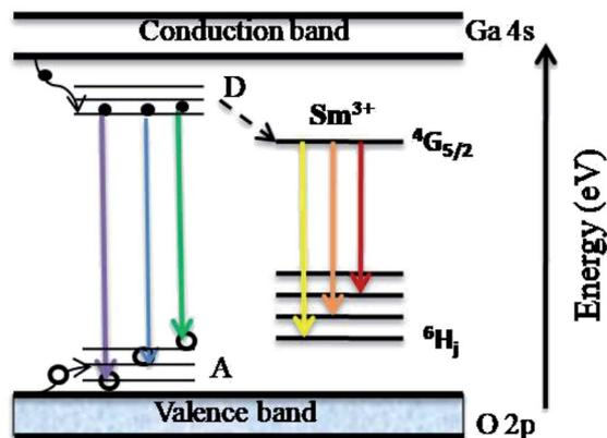
Fig. 8 Schematic representation of the charge and energy transfer processes involved in the luminescence characteristics of  $Sm^{3+}$  doped  $\gamma-Ga_{2.67}O_4$  nanoparticles. The solid spheres and open circles represent electrons and holes, respectively. D and A correspond to the defect induced formation of donor and acceptor bands, respectively.
