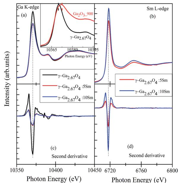
Fig. 4 (a) and (b) show the Ga K-edge and Sm L<sub>3</sub>-edge XANES spectra, respectively. The lower panels (c) and (d) are the second derivative spectra of the Ga K-edge and Sm L-edge, respectively. Inset of (a) shows a comparison of the white-line peaks of the  $\gamma$ -Ga<sub>2.67</sub>O<sub>4</sub> and Ga<sub>2</sub>O<sub>3</sub>\_900 samples.
