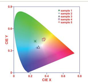
Fig. 9 CIE colour chromaticity diagram of sample 1 (pure  $\gamma$ -Ga<sub>2.67</sub>O<sub>4</sub>), sample 2 ( $\gamma$ -Ga<sub>2.67</sub>O<sub>4</sub> : 5Sm), sample 3 ( $\gamma$ -Ga<sub>2.67</sub>O<sub>4</sub> : 10Sm), sample 4 (Ga<sub>2</sub>O<sub>3</sub>\_600) and sample 5 (Ga<sub>2</sub>O<sub>3</sub>\_900).
