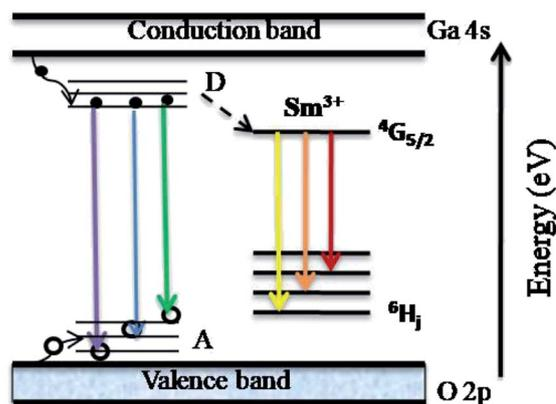
Fig. 8 Schematic representation of the charge and energy transfer processes involved in the luminescence characteristics of  $Sm^{3+}$  doped  $\gamma-Ga_{2.67}O_4$  nanoparticles. The solid spheres and open circles represent electrons and holes, respectively. D and A correspond to the defect induced formation of donor and acceptor bands, respectively.
