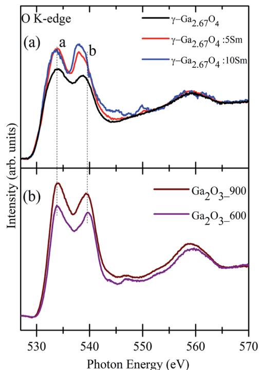
Fig. 2 (a) Normalized O K-edge XANES of (a)  $\gamma$ -Ga<sub>2.67</sub>O<sub>4</sub>,  $\gamma$ -Ga<sub>2.67</sub>O<sub>4</sub>:5Sm and  $\gamma$ -Ga<sub>2.67</sub>O<sub>4</sub>:10Sm samples and (b) O K-edge spectra of Ga<sub>2</sub>O<sub>3</sub>-600 and Ga<sub>2</sub>O<sub>3</sub>-900 samples. Dotted vertical lines on the peaks a and b indicate the energy position.
