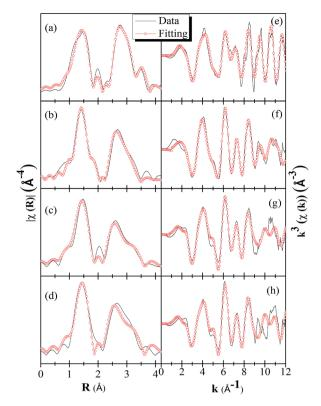
Fig. 6  $\chi(R)$  vs. R spectra of (a)  $Ga_2O_3_900$ , (b)  $\gamma$ - $Ga_{2.67}O_4$ , (c)  $\gamma$ - $Ga_{2.67}O_4$ : 5Sm and (d)  $\gamma$ - $Ga_{2.67}O_4$ : 10Sm, respectively.  $\chi(k)$  vs. k spectra of (e)  $Ga_2O_3_900$ , (f)  $\gamma$ - $Ga_{2.67}O_4$ , (g)  $\gamma$ - $Ga_{2.67}O_4$ : 5Sm and (h)  $\gamma$ - $Ga_{2.67}O_4$ : 10Sm, respectively. The spectra are not corrected for phase shift.
