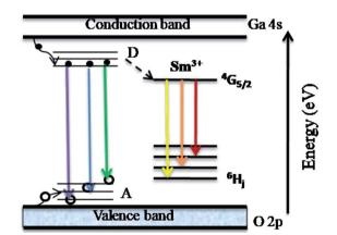
Fig. 8 Schematic representation of the charge and energy transfer processes involved in the luminescence characteristics of Sm<sup>3+</sup> doped  $\gamma$ -Ga<sub>2.67</sub>O<sub>4</sub> nanoparticles. The solid spheres and open circles represent electrons and holes, respectively. D and A correspond to the defect induced formation of donor and acceptor bands, respectively.
