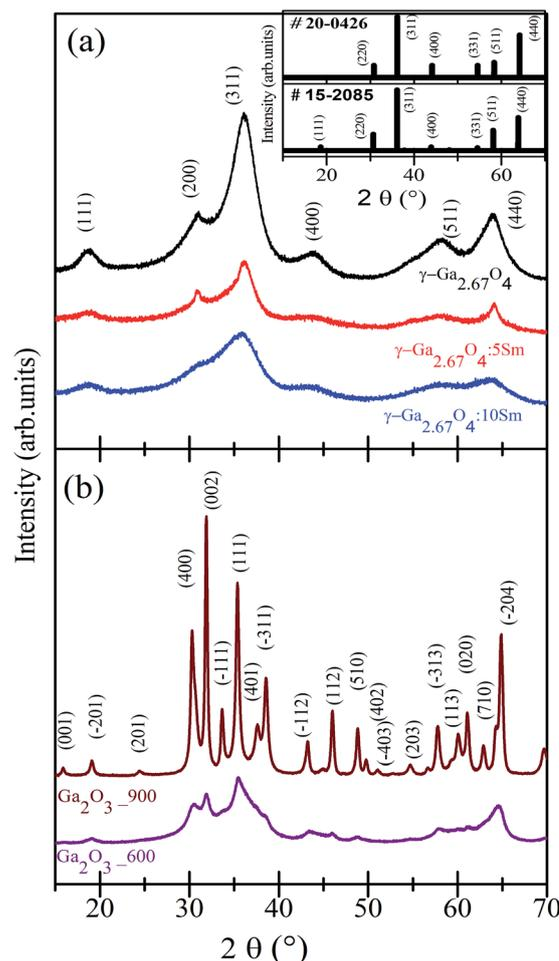
Fig. 1 (a) XRD patterns of pure and Sm doped  $\gamma$ -Ga<sub>2.67</sub>O<sub>4</sub>. (b) XRD patterns of the samples annealed at 600 °C and 900 °C. Spectra are vertically shifted for clarity of the data.
