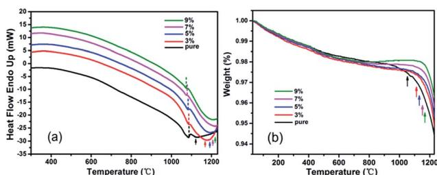
**Fig. 7** The DTA (a) and TG (b) for pure and RTP:Ta crystals.
