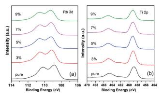
Fig. 4 High-resolution X-ray photoelectron spectra of (a) Rb 3d core level and (b) Ti 2p core level of pure and RTP:Ta crystals.
