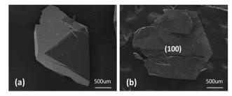
Fig. 2 The SEM observation of the morphology of (a) pure RTP and (b) RTP:Ta crystals. The (100) face was more developed after doping Ta ions
