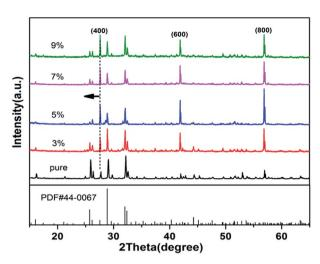
Fig. 1 XRD patterns of pure and Ta-doped RTP crystals.
