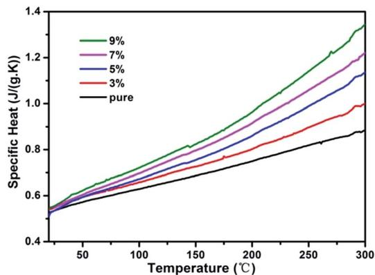
**Fig. 8** Specific heat curves of pure and RTP:Ta crystals as a function of temperature.**Table 5** Second-harmonic generation intensity of RTP:Ta crystals in relation to pure RTP crystal
