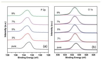
Fig. 5 High-resolution X-ray photoelectron spectra of (a) P 2p core level and (b) O 1s core level of pure and RTP:Ta crystals.
