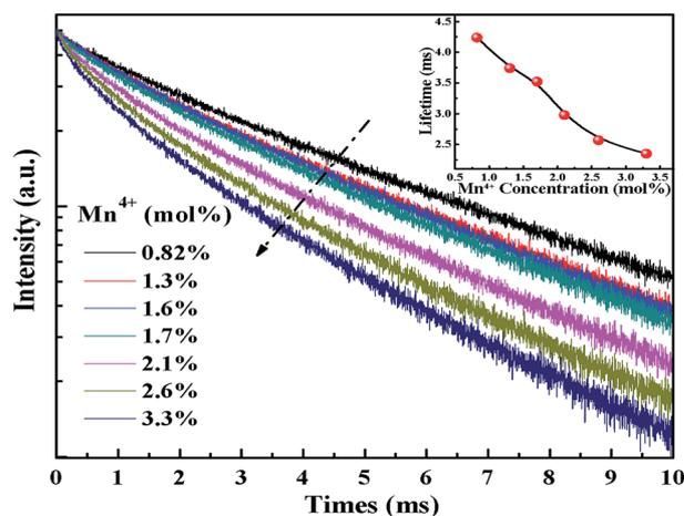
Fig. 9 Room temperature PL decay curves of  $K_2NaGaF_6$  doped with different Mn<sup>4+</sup> concentration. The inset shows the lifetimes of  $K_2NaGaF_6:Mn^{4+}$ .
