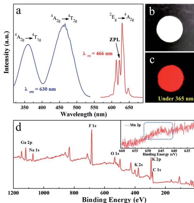
Fig. 4 (a) PLE and PL spectra (1.76 mol%  $Mn^{4+}$ ), (b) image obtained under natural light (1.76 mol%  $Mn^{4+}$ ), (c) image obtained under UV-light (1.76 mol%  $Mn^{4+}$ ), and (d) XPS spectrum of  $K_2NaGaF_6:Mn^{4+}$  (1.76 mol%  $Mn^{4+}$ ). The inset is the magnification of  $Mn^{4+}$  part of the spectrum.
