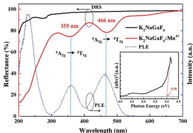
Fig. 6 DRS of the non-doped and  $\text{Mn}^{4+}$ -doped  $\text{K}_2\text{NaGaF}_6$  and PLE of  $\text{K}_2\text{NaGaF}_6:\text{Mn}^{4+}$  (1.76 mol%). The inset shows the Tauc plot for the non-doped sample.
